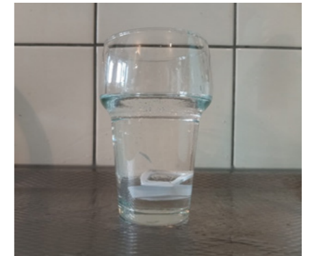
Figure E.2: Samples are placed near the bottom in a glass of glycerine at the start of the test.
