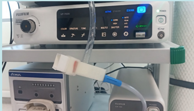
Figure 6.1.4: Low polyp trap prototype with outlet on side connected to endoscope.
