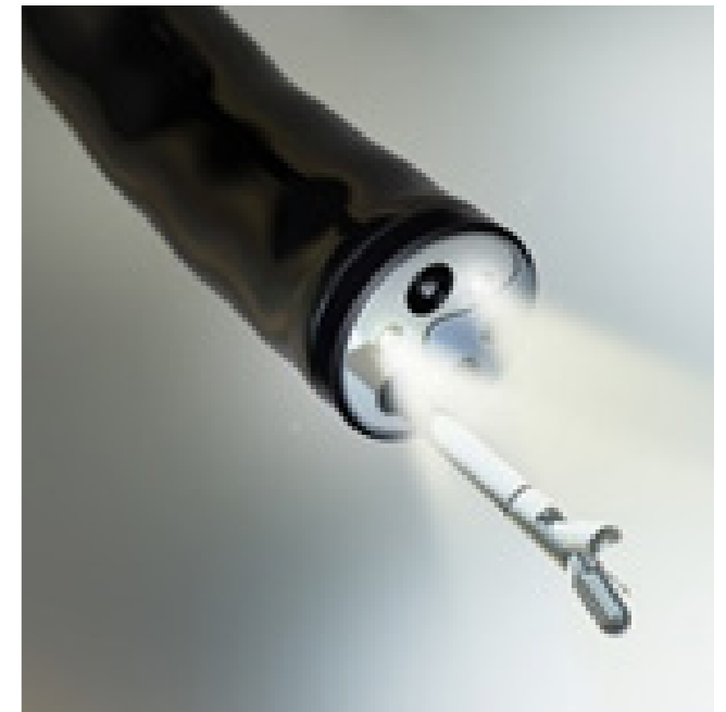
Figure 3.1.5: biopsy forceps protruding from the instrument channel of the distal tip of an endoscope.
