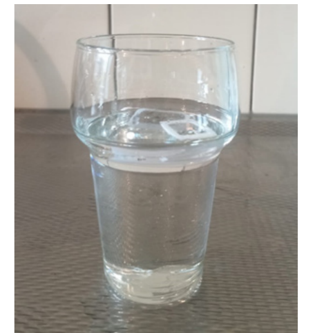
Figure E.3: Side view of float test results; polyp trap samples floating on top of the glycerine.
