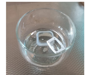
Figure E.4: Top view of float test results; polyp trap samples floating on top of the glycerine.
