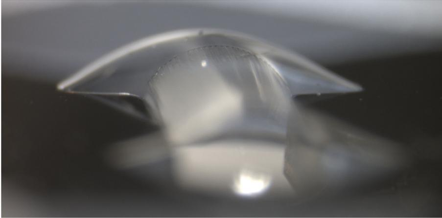
Figure 43: Image obtained by the microscope of the dogbone membrane including grooves. Notice that in the centre region the membrane seems to leave the edges under a considerable angle. The effect of the clamped edges appears to be extremely small.
