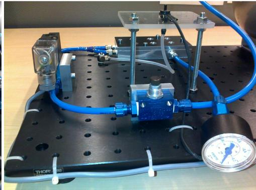
Figure 91: Manual analogue flow regulator (centrally situated in the image, blue box with grey turning wheel). The flow regulator is adjusted until the right absolute peak pressure is obtained (read out on computer screen).
