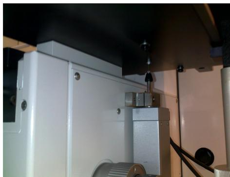
Figure 67: The measurement of the table height (and thus deflection) when focussing visually, is done by a sensor situated underneath the table.
