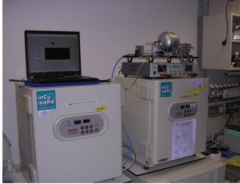
Figure 95: The entire experimental setup. The chip-holder is placed in the incubator situated underneath the experimental setup's mechanical part. Control and readout is done by means of a laptop with Labview.
