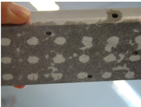
Figure 105: Bottom view of the chip-holder, the contact with another metal in the incubator initiated corrosion.
