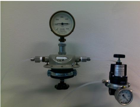
Figure 64: Analogue regulated compressed air, to fill the pressure box.
