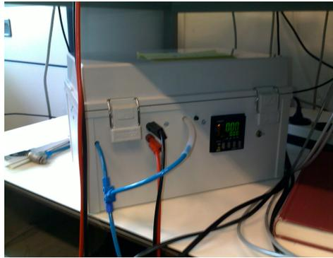
Figure 63: Pressure box, to generate a constant pressure.
