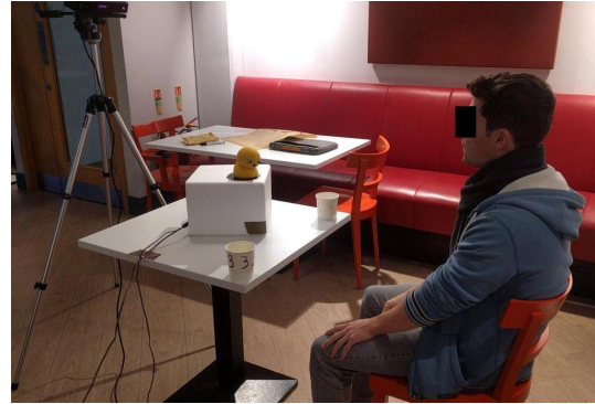
Figure 1: Experimental setup of the Active condition: the participant is seated at a dining table with two bowls with identical chocolates; the robot is placed on the table at an equal distance from the bowls, performing non-verbal behaviors to influence participant's food choice.
