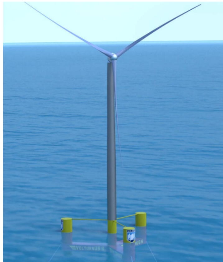
Figure 1.3: UMaine VoltturnUS-S platform is designed to support the IEA-15-240 RWT system. This type of structure is used for the case study [2]
