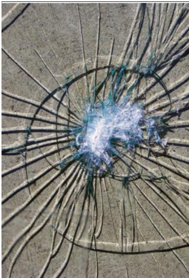
Image 33 - Break pattern of glass. Wurm, 2017.
