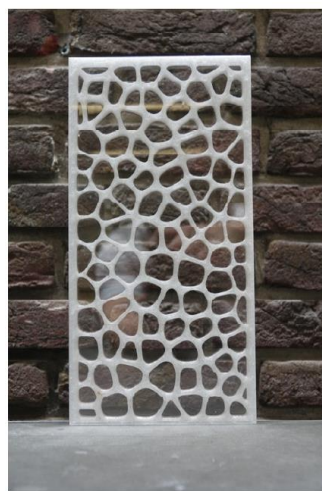
Image 3 - 8 mm core thickness. 1 mm thin glass (Neeskens, 2018)
