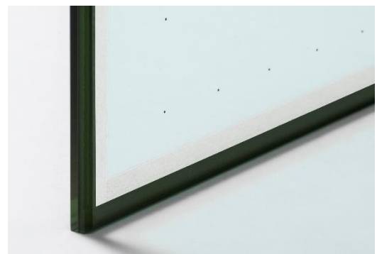
Image 15 - VIG panel. 2 layers of 3mm glass with cavity of 0,1mm. Photo: AGC
