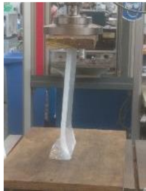
Image 113 - Standard pattern 1 deformation due to compression. Own image.
