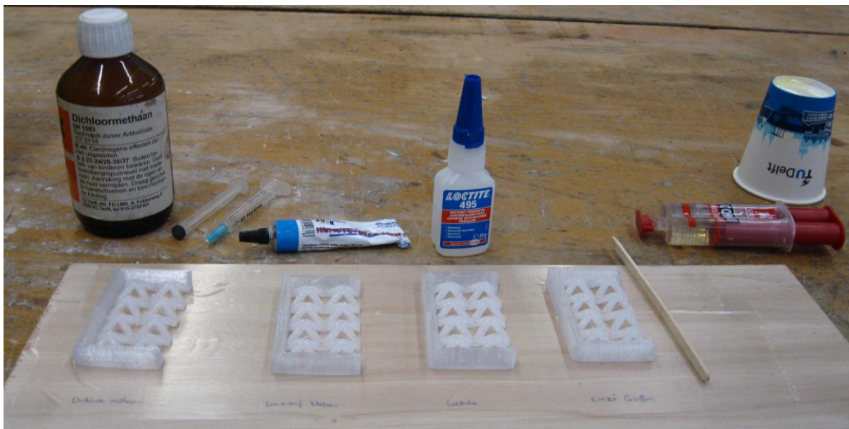
Image 63 - Different types of bonding materials. From left to right: Dichloromethane, Kunststoffkleber, Loctite 495, Two-component Griffon. Own image.
