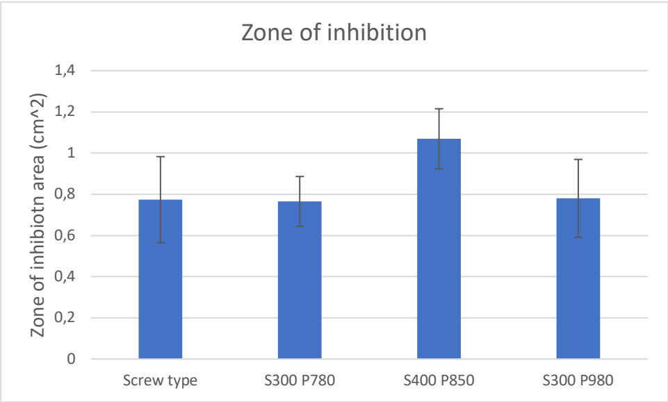
Zone of inhibition of dental implants. This test indicates the zone of inhibition of the dental implants against MRSA. Bars indicated the standard deviation of the results (n=3 for all implants). In this test the porous implants could not lie flat in the agar.
