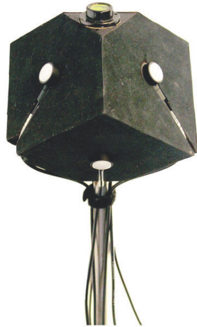
Figure 1. Our cubic illumination meter, built with commercially available components on the basis of a laser-cut cube base (see Appendix for additional materials to build this base). Note: our cubic illumination meter has six large faces and two small faces. The small face on the top was cut to place a spirit level, and the small face on the bottom was cut to fix the cubic meter onto a metal stick.
