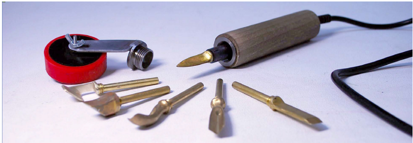
Figure 150: tool tips for welding Scrap plastics (Lopez Pradas, 2013)
