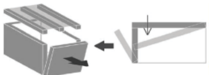
Figure 23: Discontinuity of walls leads to out-of-plane tipping and floor falling, source: Arup, 2013
