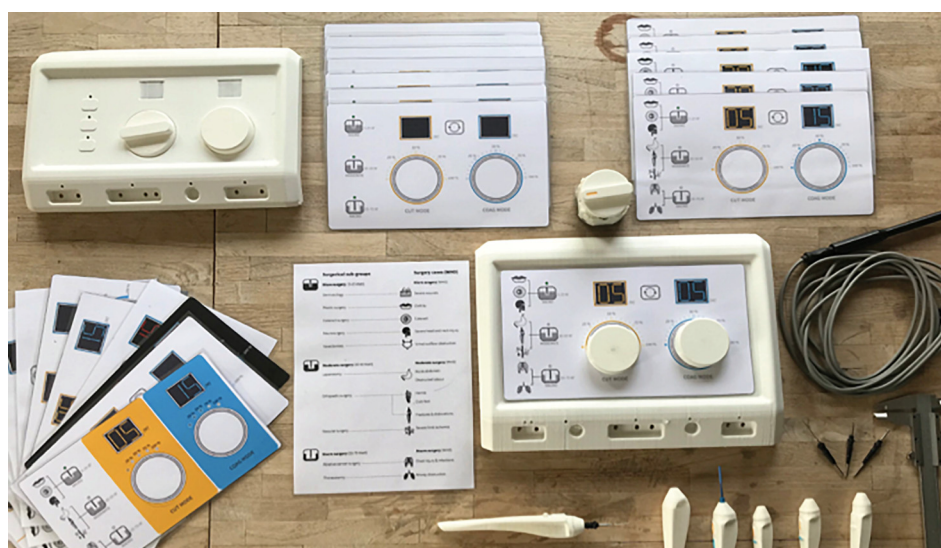
Fig. 1 Demonstrator designs of the ESU interface and the monopolar handheld that were evaluated by 19 surgeons and 2 BMETs working in Kenya (study 4, Table 1)
