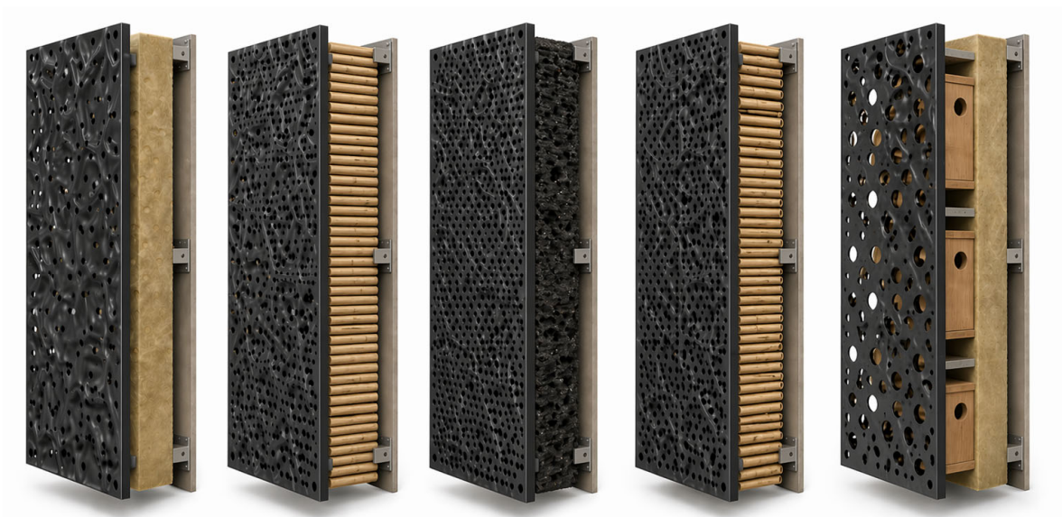
Figure 97: Potential design variations with different back structures; from left to right: mineral wool, reed, foamed furan resin, reed higher density, nature inclusive (e.g. birds) (source: Author)
