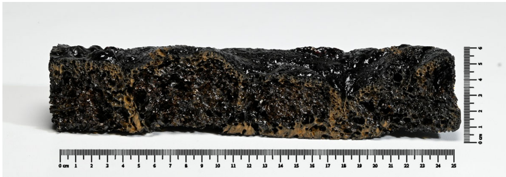
Figure 41: S9 foamed material (source: Author)
