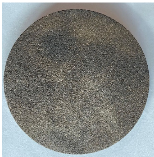
Figure 47: Sanded Cork Furan Material D (source: Author)
