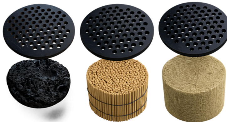
Figure 74: Different set-up configurations for the perforated external material (20%) and S3 (left), 100mm reed (middle) & 100mm mineral wool (right) (source: Author)
