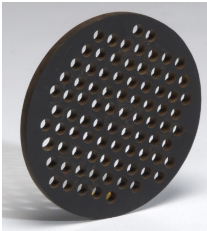
Figure 43: Perforated biocomposite 8040 Hemp Fire (20% perforation rate)
