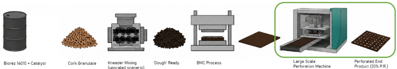
Figure 98: Current production process at NPSP for pressed biocomposites and a possible upscale perforation device added (source: Author)
