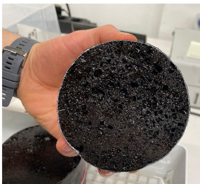
Figure 109: WA (Water absorption) test close-up (source: Author)
