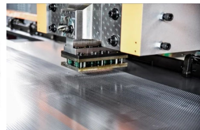
Figure 21: Perforations on an industrial scale with the (punch method) (source: IndiaMART, n.d.)
