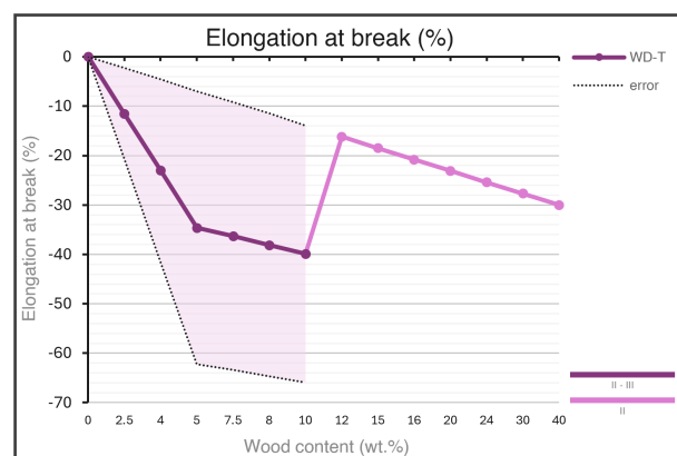
Figure A.178. Combined effect of thermally-treated wood dust (WD-T) content in PLA matrix on the elongation at break (relative % compared to neat PLA). Adapted from II. Gregorova et al., 2011 [46]; III. Ayırlmis et al., 2021 [8].
