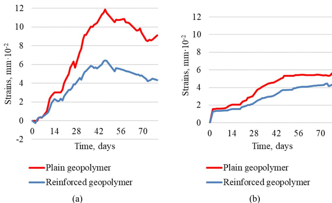
**Figure 6: Shrinkage (a) and creep (b) strains**
