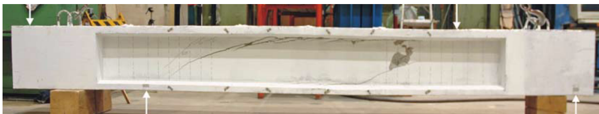
Figure 3-10: Failure of the beam LB11 [13]; A_s = 934\text{mm}^2 , N = -809\text{kN} , V_u = 142.8\text{kN}
