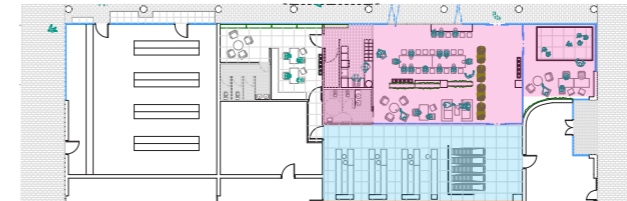
Figure 7.1.6: Lidl entrance refurbishment, with entrance area (pink colour), cash area (blue) and commercial area (brown).
