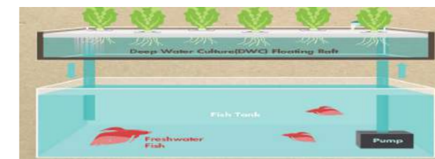
Figure 4.5.1.4: DWC aquaponics system (DWC) (Source: Desima, 2016).
