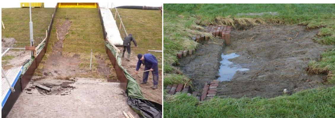
**Figure 5 Scour hole development at the toe with a hidden brick path (left: overview; right: detail)**
