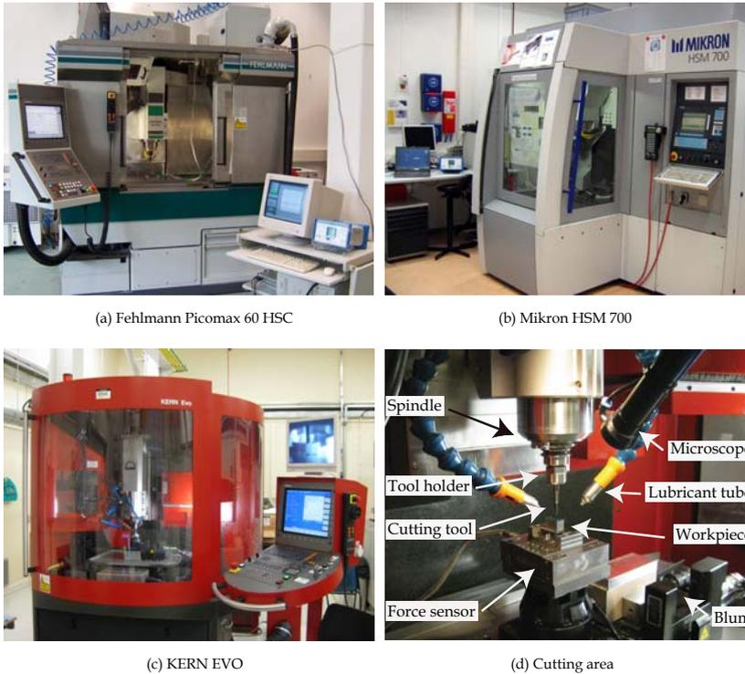
**Fig. 3.6:** Machine tools used in experiments.
