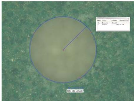
**Fig. A.2:** Measure the radius of the drilled hole by an optical microscope.
