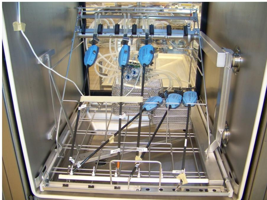
Figure 6.6: test setup configuration II. The da Vinci mobile unit placed in a washer-disinfector. Three Endowrist instruments were connected as in real situation and three instruments are connected to the measurement system. The measurement system was placed between the instruments and the mobile unit.
