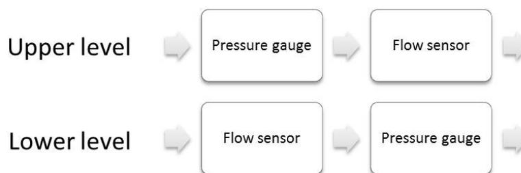
Figure 8.3: schematic view of the configuration of the measurement system. The upper level of the channels first consist of a pressure gauge and then a flow sensor and for the lower level the configuration is reversed.
