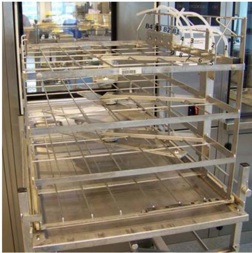
(a) Mobile unit Miele E909 with 9 small adapters and 4 large adapters
