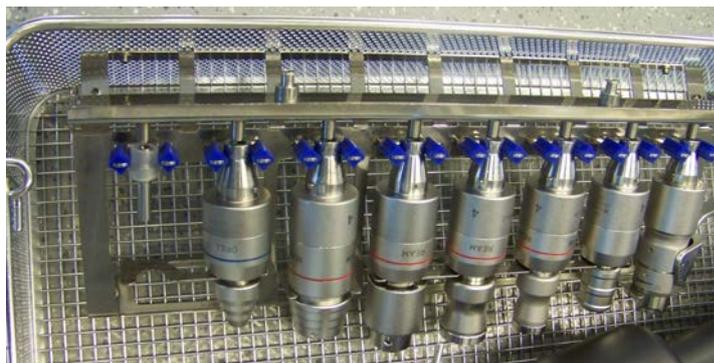
Figure 2.7: an insert fixed in an instrument tray with 8 adapters, allowing eight instruments to be connected to this insert. The insert is able to fix and rinse eight hollow drilling attachments. The attachments are placed close to the adapter, but there is no contact between instrument and adapter, this connection is called a contactless connection.
