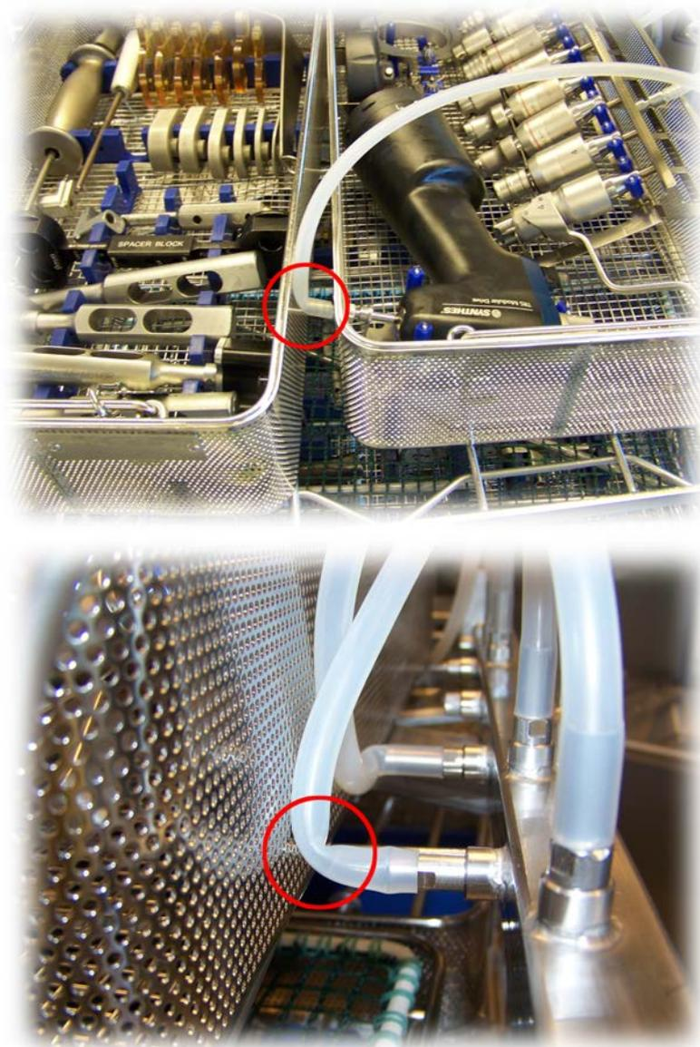
the mobile unit has multiple adapters to connect hollow instrument for rinsing inside. The connection between the adapter and the instrument consists of a flexible silicone tube. A flexible tube is not always convenient, a kinked tube leaves little fluid...
