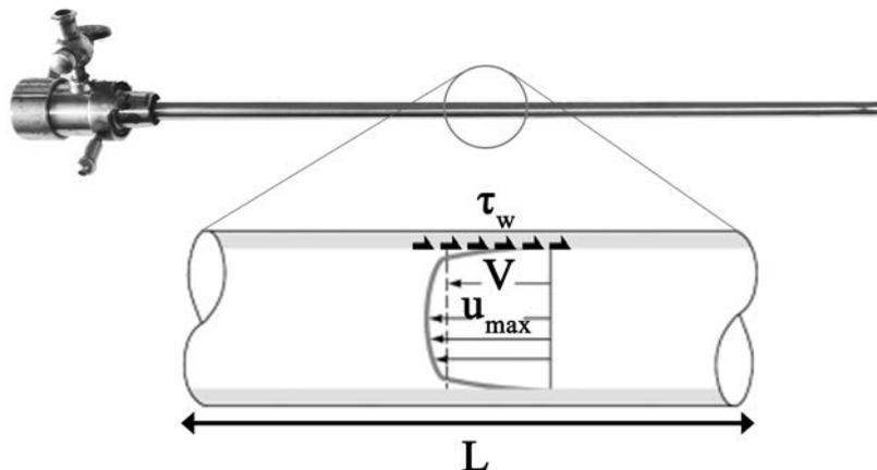
Figure 3.1: a schematic view of the flow in a hollow instrument. The flow streams from right to left. The flow applies a force to the wall, this force is called 'wall shear stress'. It is desired that the wall shear stress is as high as possible to realize an optimal cleaning capacity.
