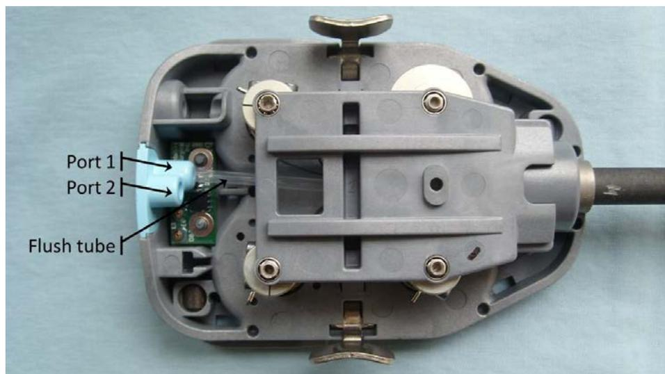
Figure 6.4: inside housing of an Endowrist instrument. The instrument consists of two irrigating ports, the main port irrigates the inner distal end via a flush tube and the second port is for rinsing the housing of the instrument. The second port irrigates only the inside of the housing therefore no tube is connected. Thus there is much less resistance, which leads to a higher flow.
