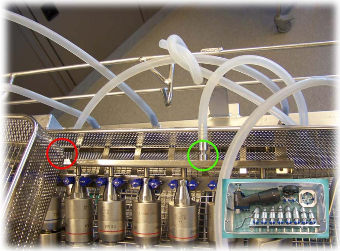
a tray with hollow biodrive attachments. The distribution block is developed specially to ensure that each attachment can be rinsed on the inside. The distribution block has two inlet ports to build up pressure and get enough flow for the eight attachments. The attachments are placed correctly before the adapter and the inlet adapters are connected to the mobile unit. It seems to be a correct situation. However, they thought it is sufficient to connect one inlet adapter...
