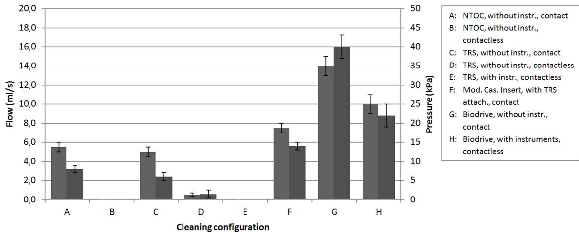
Figure 5.4: the mechanical performances - expressed as flow and pressure - for the different cleaning configurations.
