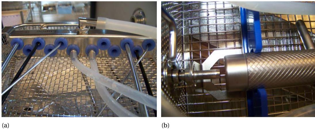
Figure 5.1: a contactless adapter vs. a contact adapter. A) contactless adapter: the instrument has to be placed near to the injector nozzle. B) contact adapter: the instruments are pushed into the silicone holder.
