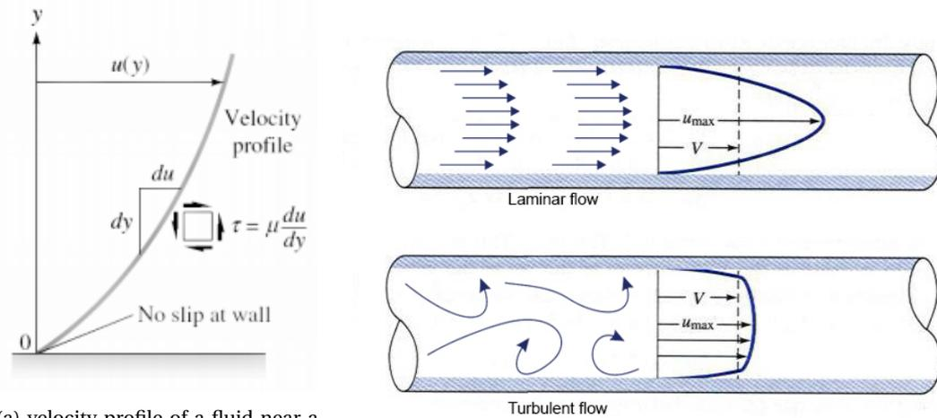
(a) velocity profile of a fluid near a layer. At the wall the fluid velocity is relative to the wall (no-slip condition), if the wall has no velocity than velocity profile, a turbulent flow (Re > 4000) is characterized by a chaotic the velocity at the wall is also zero. (b) a laminar flow (Re < 2300) is a tidy layered flow and has a parabolic velocity profile, a turbulent flow (Re > 4000) is characterized by a chaotic flow and the velocity profile is smoother.
