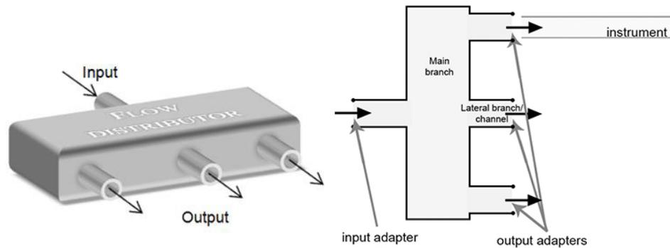
Figure 4.1: schematic view of an insert. The working principle is like a manifold: the input flow is distributed among multiple outputs. The input adapter of the insert is connected to a mobile unit and instruments can be connected to the output adapters.
