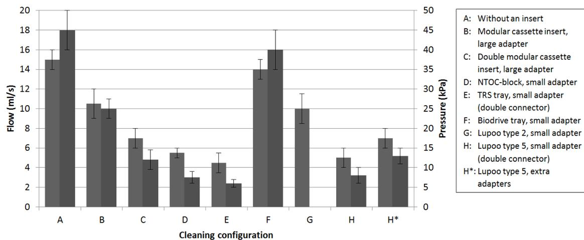
Figure 4.8: flow and pressure in the adapters for several cleaning configurations.
