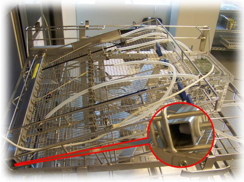
the number of hollow instruments are increasing very fast. The standard equipment of a washer-disinfector has too few connecting possibilities. Therefore inserts are used with much more possibilities for connecting hollow instruments. These inserts can apply sufficient flow and pressure to rinse thirteen instruments, although the end stopper should not be missing...
