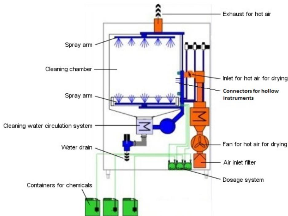
Figure 1.5: simplified diagram of a washer-disinfector. Spray arms are placed at the bottom and the top of the cleaning chamber. Adapters for hollow instruments are at the side. [5]
