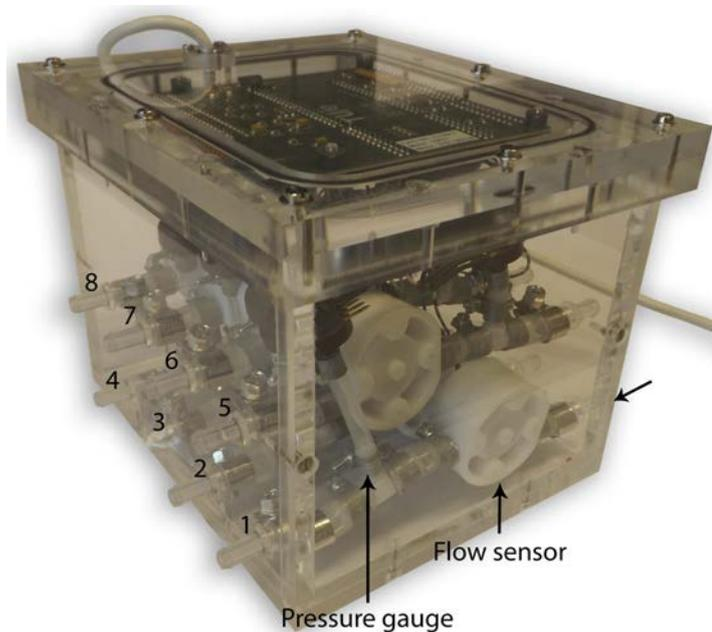
Figure 2.9: Measurement system, developed by *Causa BV*, Eindhoven, The Netherlands. The system is able to measure the flow and pressure in eight separated channels.
