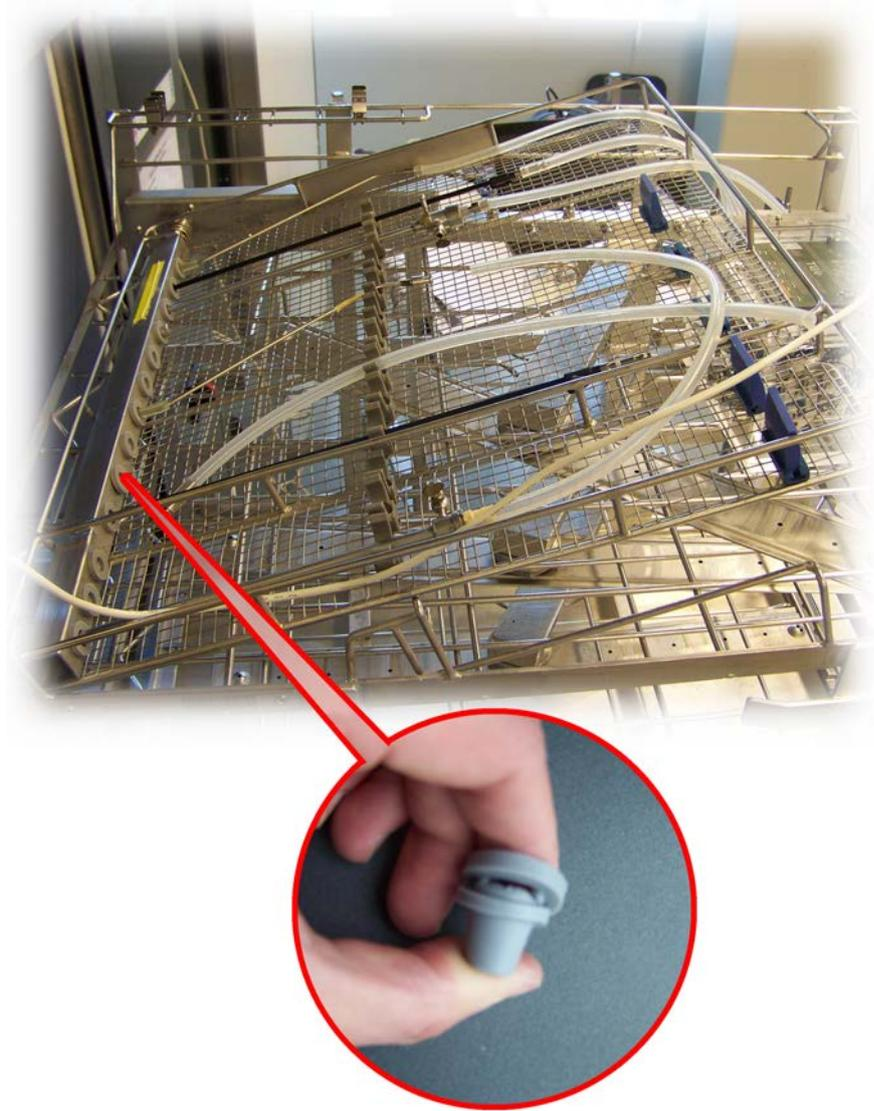
cracks may arise from the insertion and removal of instruments in the silicone holders. Cracks in the silicone holder cause leaks and result in flow and pressure loss. Maintenance is of great importance!
