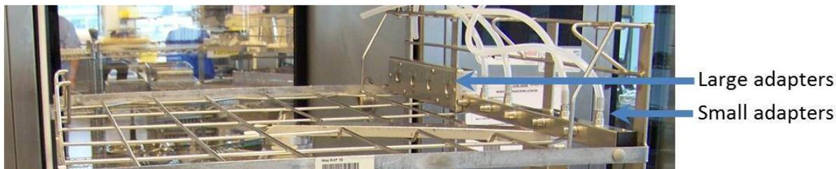
Figure 2.5: close-up of the top level of a mobile unit with an adapter block. The adapter block has nine small adapters and four large adapters. Some inserts have to be connected to the large and others to the small adapters. Hollow instruments or injector nozzles can also be directly connected to a small adapter. The adapters of the mobile unit are fed by the central pumping system of the washer-disinfector.
