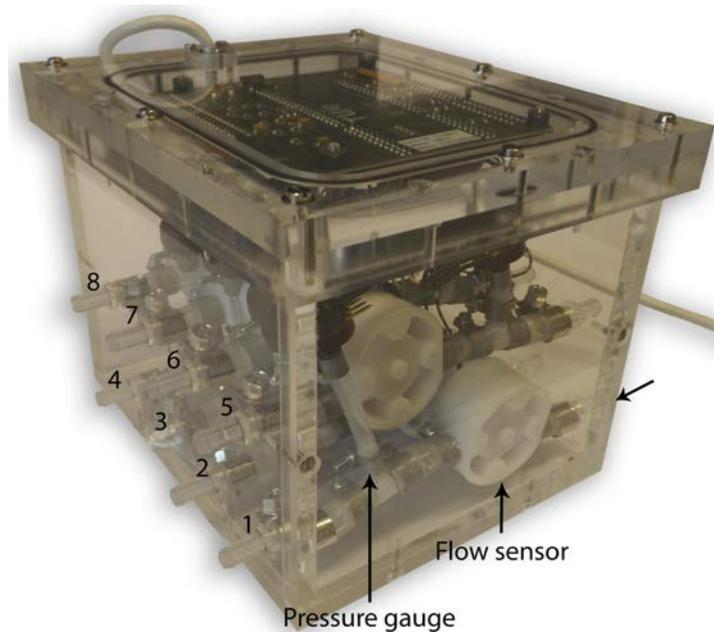
Figure 8.2: measurement system consists of two levels with four measurement channels each. A measuring channel consists of a flow sensor and a pressure gauge. The configuration of the upper level is reversed by the configuration of the lower level. The lower level first has a flow sensor and then a pressure gauge, and for the upper level is it reversed.
