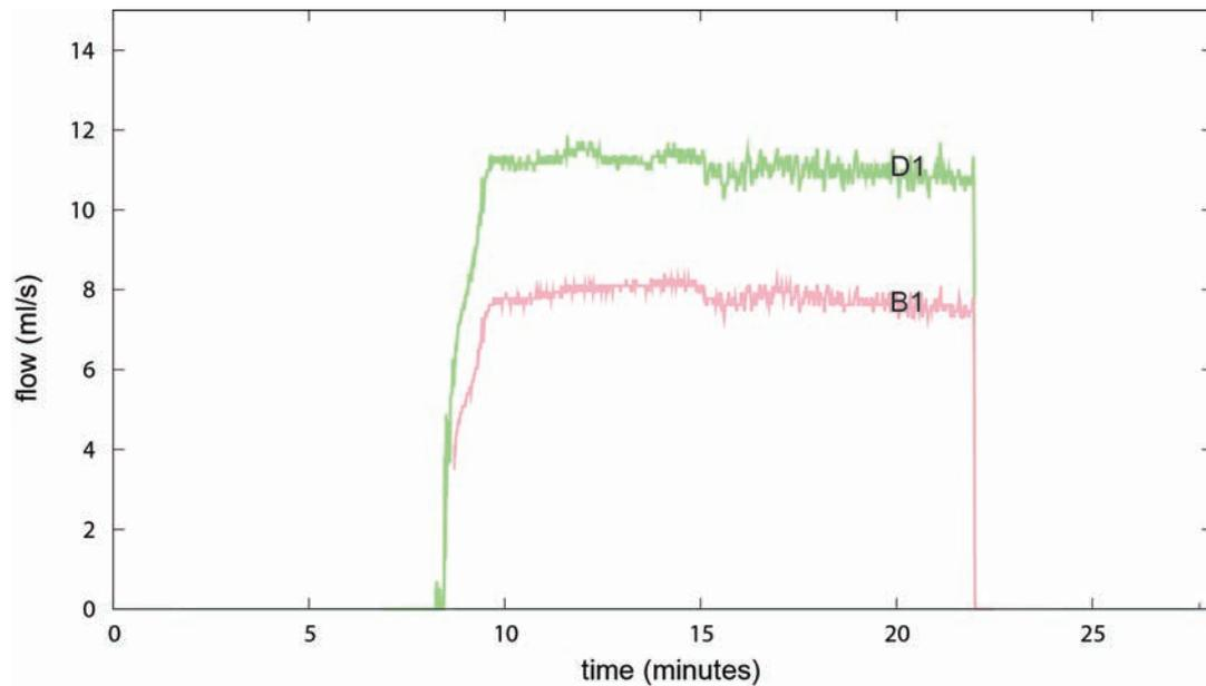
Figure 3.4: the flow through the dummy instruments during a cleaning process.
