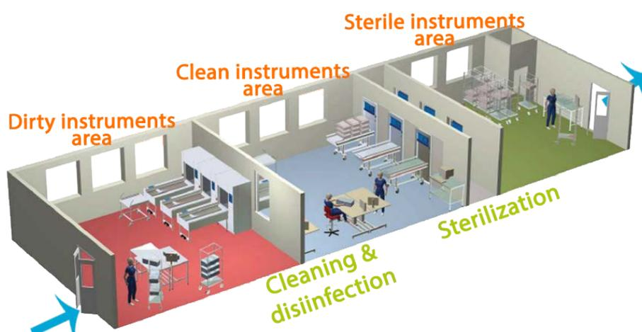
Figure 1.2: reusable instruments were reprocessed at a Central Sterile Supply Department. This department consists mostly of three separate parts. In the first room the instruments were dirty and contaminated. After the cleaning and disinfection process the instruments were clean. In the last phase the instruments were sterilized, at the end the instruments were clean and sterile.
