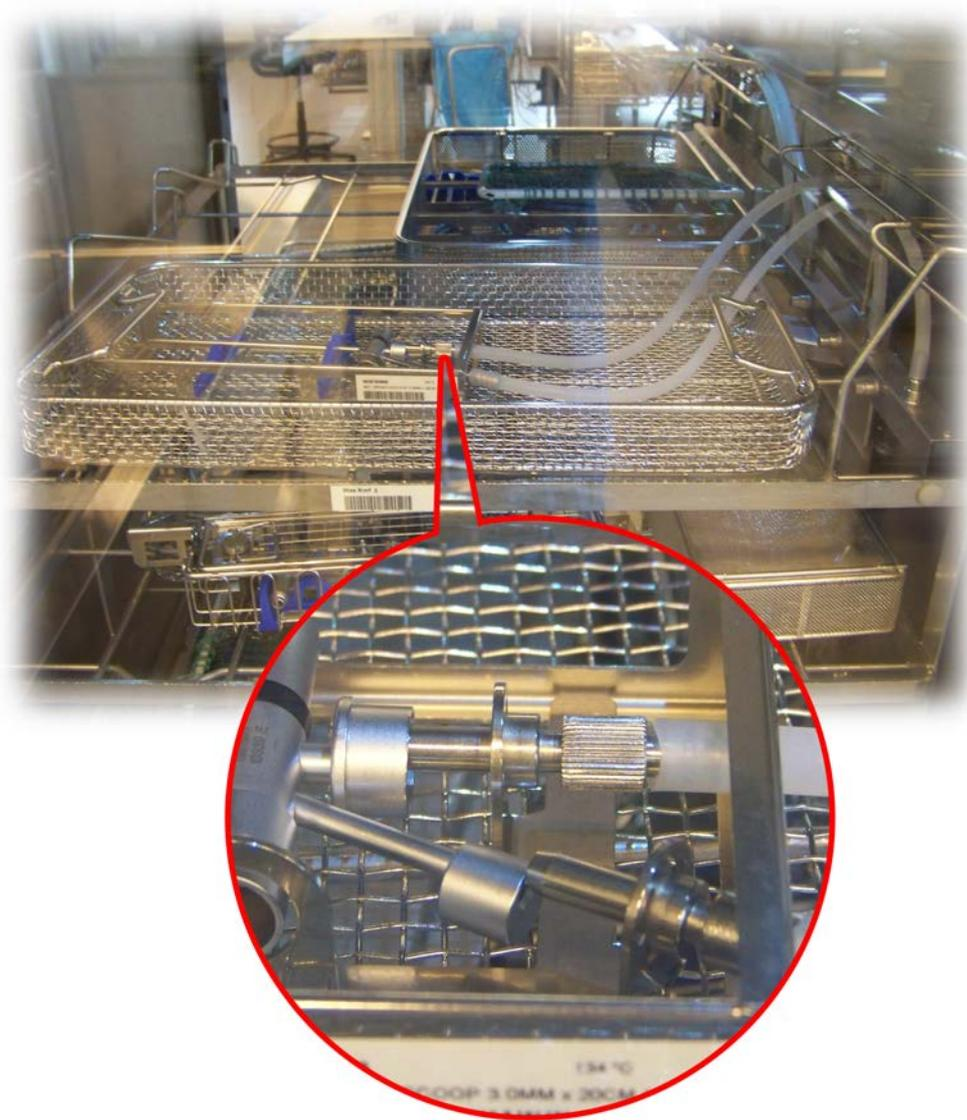
a tray with two hollow instruments, the adapters are connected correctly to the mobile unit. But if we look more in detail then we see that the instrument is not placed in front of the nozzle...
