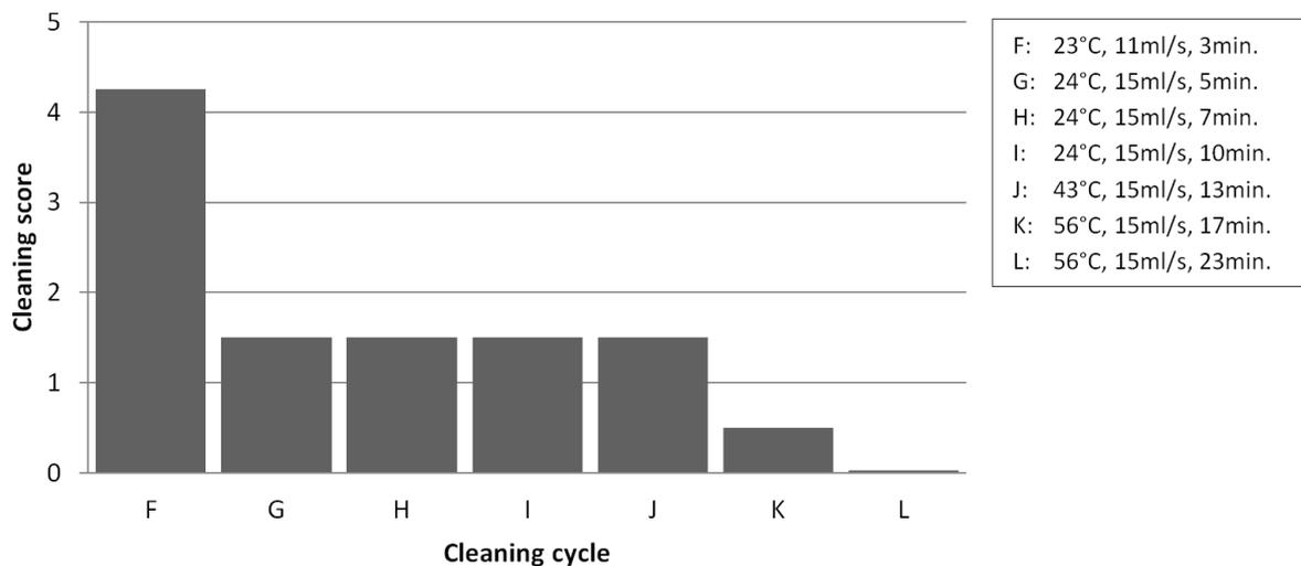
Figure 7.4: the test soil was evaluated during the cleaning process (Table 7.2).
