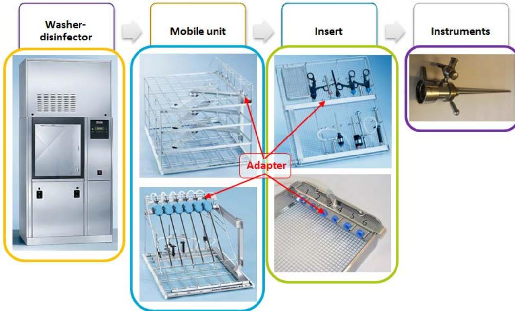
Figure 8.4: an overview of the chain of elements. A mobile unit can be rolled into a washer-disinfector. Instrumentsets are placed on a mobile unit and a mobile unit has adapters for hollow instruments to connect them to the pumping system of the WD. Sometimes an insert is connected to the mobile unit and the insert has more adapters or adapters specifically for special hollow instruments.
