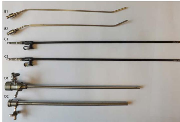
Figure 2.8: six dummy instruments. These instruments were used in the test with hollow instruments. The dummy instruments can be categorized in three types based on their design: short plus curved, long plus straight and short plus straight.
