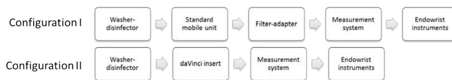
Figure 6.2: Overview of both test configurations. In the first configuration the filter-adapter was tested. The filter-adapter was connected to a standard mobile unit. The measurement system was placed between filter-adapter or the da Vinci mobile unit and the Endowrist instruments.
