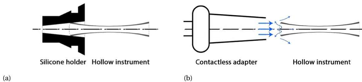
Figure 5.2: a) a schematic view of a contact adapter. An instrument is pushed into a silicone holder, therefore the tip of the instrument is enclosed by the holder and cannot be cleaned very well. b) a schematic view of flow loss in the open contactless connection between an adapter and the instrument.
