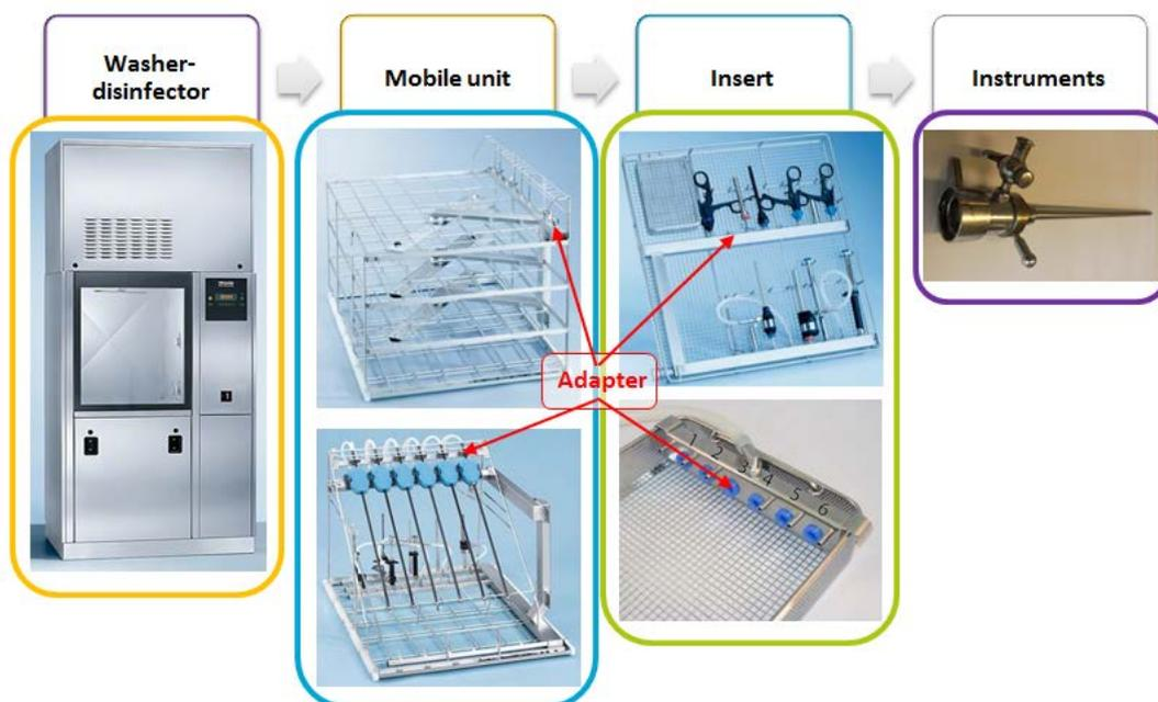
Figure 2.1: an overview of the chain of elements. A mobile unit can be rolled into a washer-disinfector. Instrumentsets are placed on a mobile unit and a mobile unit has adapters for hollow instruments to connect them to the pumping system of the WD. Sometimes an insert is connected to the mobile unit and the insert has more adapters or adapters specifically for special hollow instruments.
