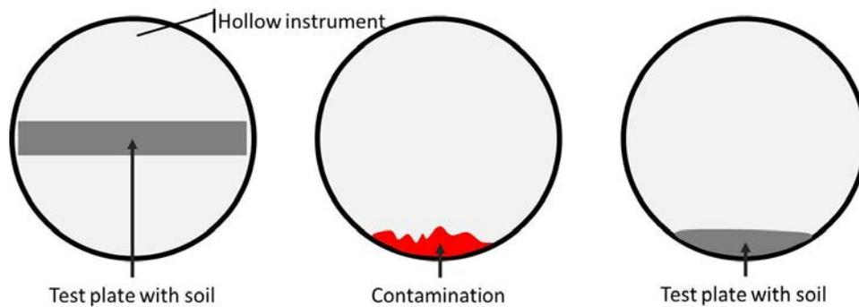
Figure 7.5: a cross-section of the test instrument with the test plate in the center, a contamination fixed at the wall of a hollow instrument and a test plate to the wall of an instrument.
