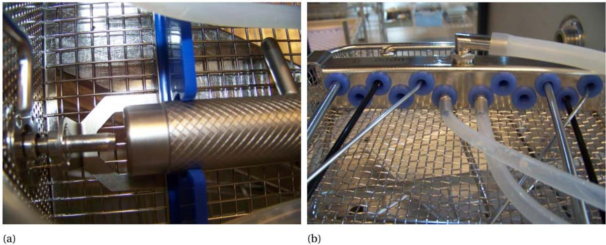
Figure 4.4: a contactless adapter vs. a contact adapter. A) contactless adapter: the instrument has to be placed near to the injector nozzle. B) contact adapter: the instruments are pushed into the silicone holder, allowing the instrument tip to be fully enclosed.
