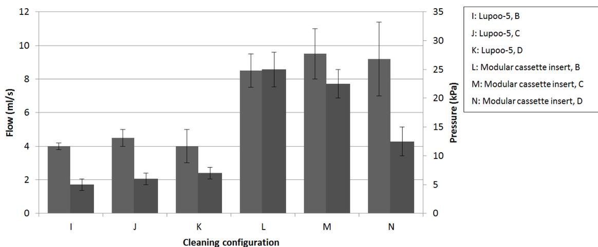
Figure 4.9: flow and pressure in instruments connected to respectively the Lupoo insert (configuration I, J, K) and the modular cassette insert (configuration L, M, N).
