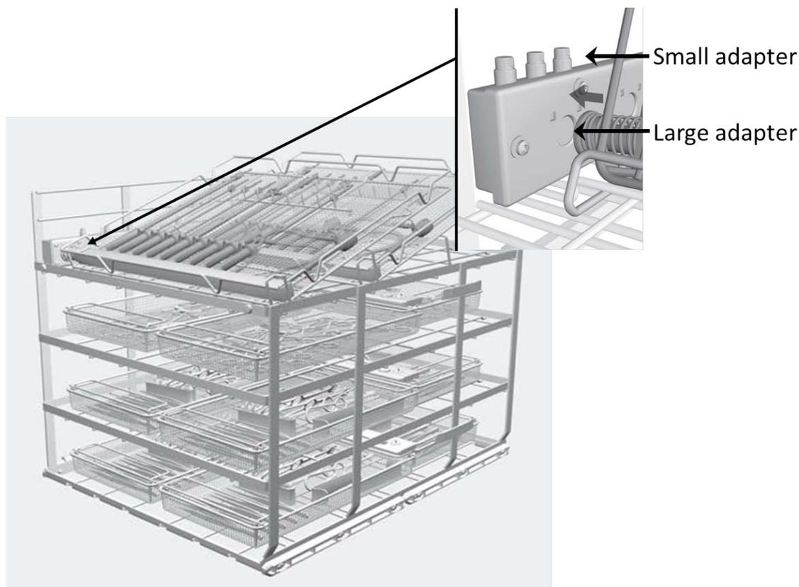
Figure 4.3: a standard mobile unit. The mobile unit can be placed in the chamber of a washer-disinfector. Instrument trays can be placed on the levels of the mobile unit. An adapter block is placed on the top level of the mobile unit. The adapter block can be used to connect inserts and hollow instruments. There are large and small adapters. The small adapters are suitable to connecting inserts or hollow instruments. The large adapters are suitable for special inserts.
