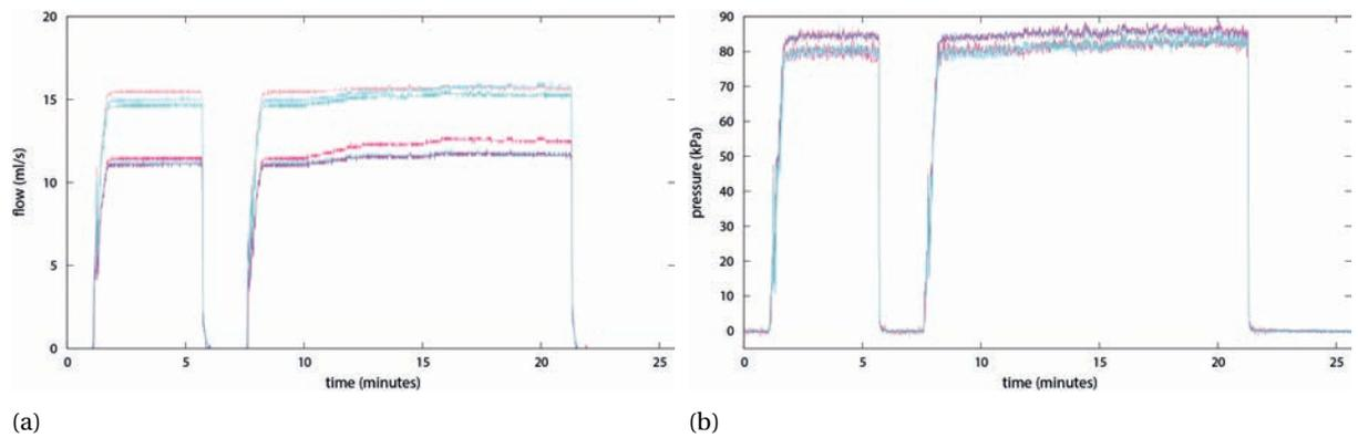
Figure 6.3: flow and pressure results of configuration II with three Endowrist instruments.
