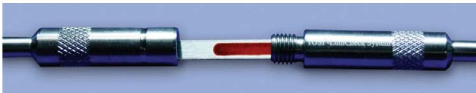
Figure 7.1: TOSI LumCheck. The LumCheck is a dummy instrument to imitate hollow instruments. A plate with a test soil is placed in the channel of the LumCheck. The test soil is composed of blood components. After the cleaning cycle the test soil has to be assessed visually. An optimal result indicates that the test soil is completely dissolved, no test soil residuals are left.
