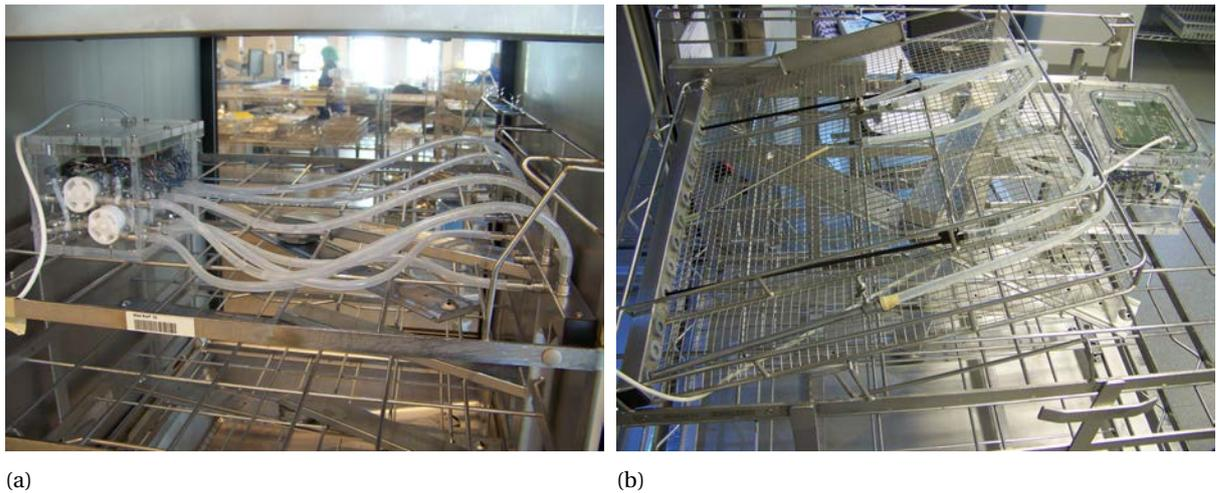
Figure 4.7: a) test setup of cleaning application A, without an insert. The measurement system was connected directly to the mobile unit. b) Test setup of cleaning configuration L, M and N with the modular cassette insert. Instruments were connected to the insert and the output of the instrument was connected to the measurement system, so flow and pressure through the instruments were measured.
