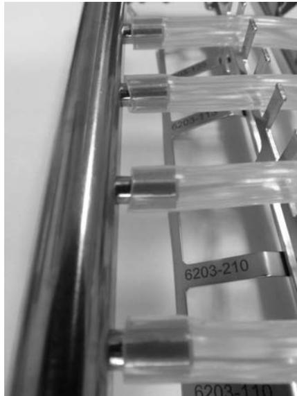
Figure 4.5: the test setup of an insert with contactless adapters. For the measurement the inserts were considered as contact adapters: a tube of the measurement system was pushed over the injector nozzles, allowing the nozzle to be fully enclosed.
