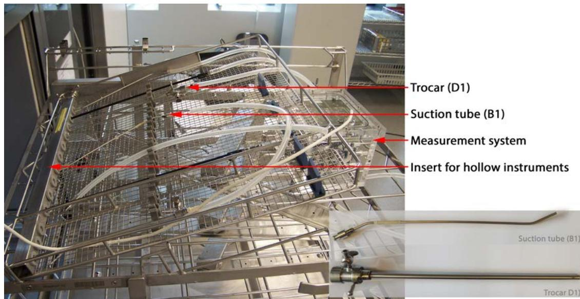
Figure 3.3: test setup consisting of instruments that are connected to a cleaning application on a mobile unit for rinsing of the inside of the instruments.
