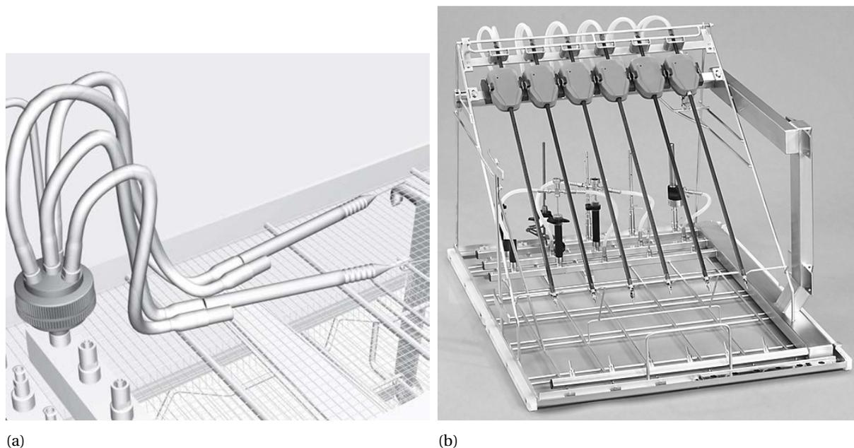
Figure 6.1: a) Filter-adapter E478/1 with four connectors for rinsing MIS instruments. The inlet of the adapter can be connected to a standard mobile unit. b) da Vinci mobile unit E928 with twelve adapters for rinsing of six Endowrist instruments. The da Vinci mobile unit can be placed directly in the chamber of a washer-disinfector.
