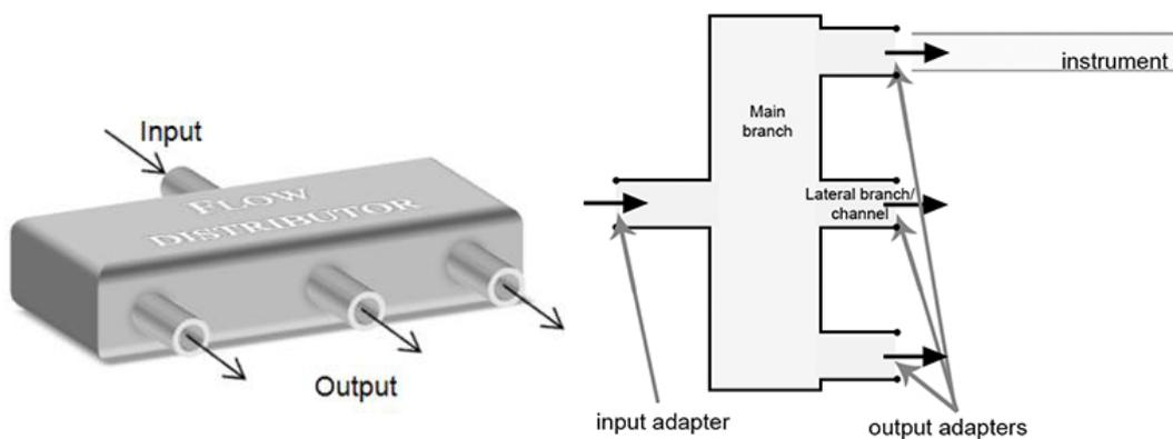
Figure 8.5: schematic view of an insert. The working principle is like a manifold: the input flow is distributed among multiple outputs. The input adapter of the insert is connected to a mobile unit and instruments can be connected to the output adapters.
