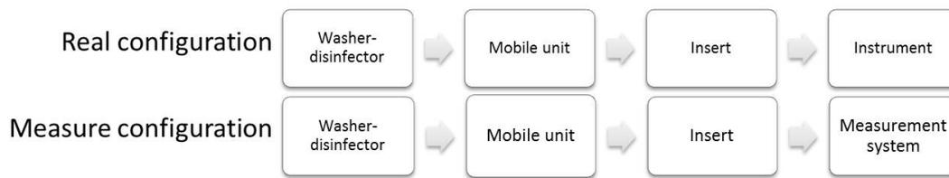
Figure 5.5: schematic view of the real configuration compared to the measure configuration. For a good interpretation of the measure results it is important to know the pressure drop of the measurement system relative to an instrument.
