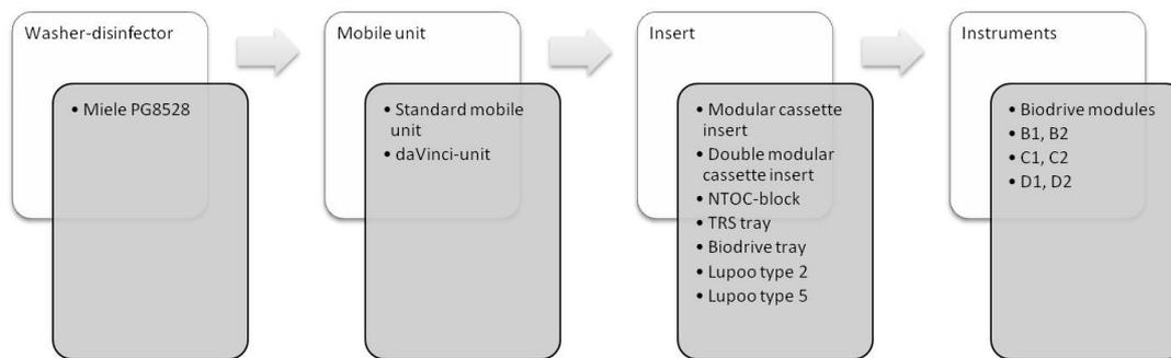
Figure 2.3: an overview of the chain of elements. A mobile unit can be rolled into a washer-disinfector. Instrument sets are placed on a mobile unit and a mobile unit has adapters for hollow instruments to connect them to the pumping system of the WD. Sometimes an insert is connected to the mobile unit and the insert has more adapters or adapters specifically for special hollow instruments.
