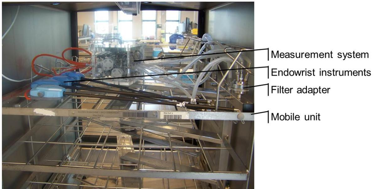
Figure 6.5: test setup of configuration I. The filter adapter was connected directly to a mobile unit and the outlet tubes of the adapter were connected to the measurement system. The four original tube-connectors of the filter-adapter were connected to the output channels of measurement system and the main port of an Endowrist instrument.
