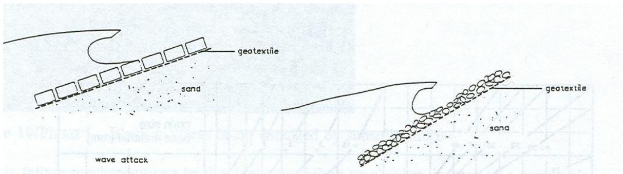
Figure 2.9 Examples of structures in which geometrically sandtight structures are necessary (Source: Klein Breteler & Bezuijen, 1998)
