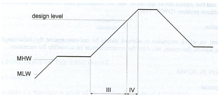
Figure 2.20 Hydraulic loading zones on riverdyke with high foreshore (Source: Van Herpen, 1998)
