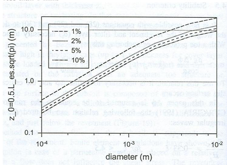
Figure 2.12 Influence of several parameters on  $z_0$  (Source: Klein Breteler & Bezuijen, 1998)
