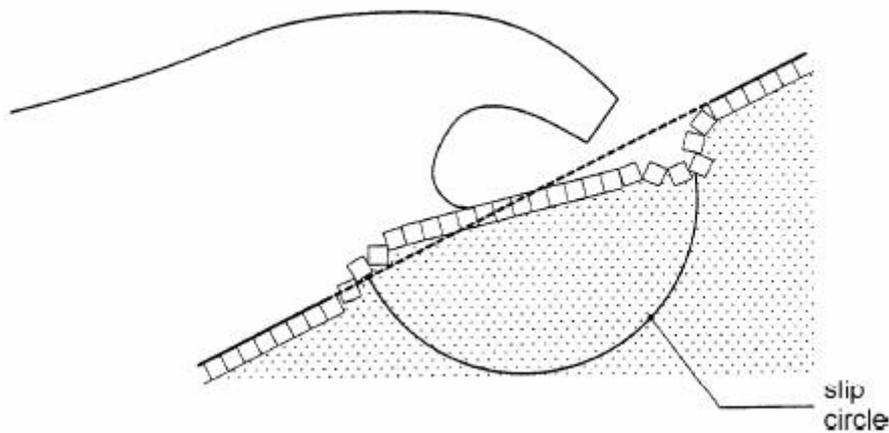
Figure 2.32 Schematised development of S-profile and possible local sliding in the base (Source: Klein Breteler et al., 1998)
