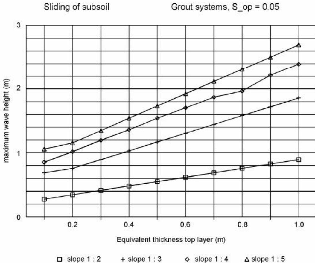
Figure 2.33 Geotechnical stability, design diagram for grouted systems and  $H_s/L_{op} = 0.05$  (Source: Klein Breteler & Pilarczyk, 1998)
