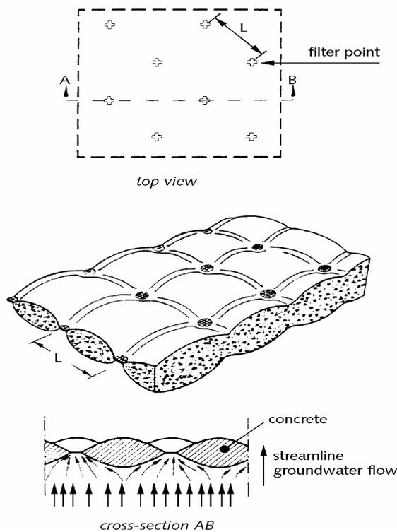
Figure 2.34 Principles of permeability of Filter Point Mattress (Source: Klein Breteler & Pilarczyk, 1998)
