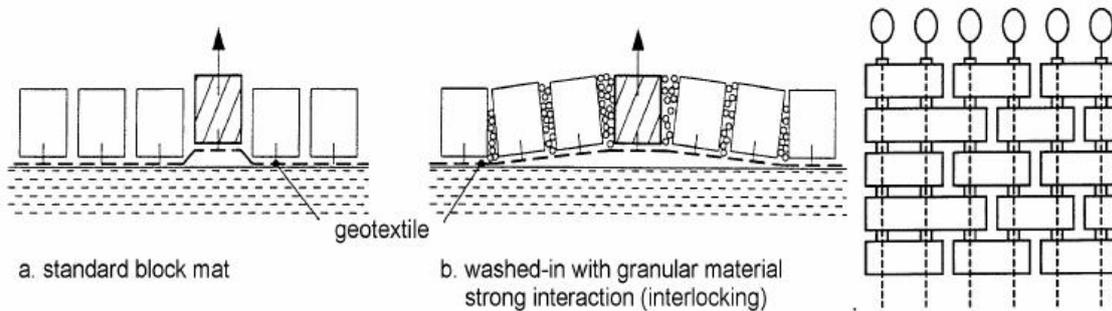
Figure 2.30 Example of block mats (Source: Klein Breteler et al., 1998)
