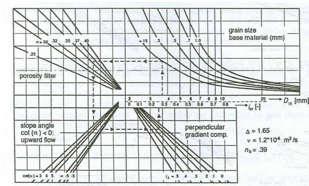
Figure 2.10 Calculation rules for critical gradient  $i_{cr}$  for granular filter on sand (Source: Klein Breteler & Bezuijen, 1998)
