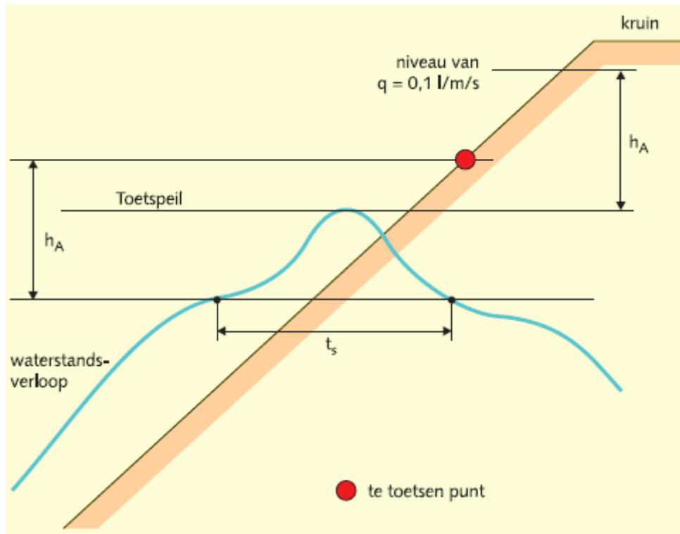
Figure 2.15 Determination of duration of loading in wave run-up zone  $t_r$  (Source: TAW, 2004)
