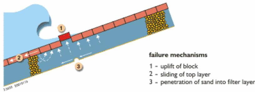
Figure 2.7 Failure mechanisms modelled in ANAMOS
