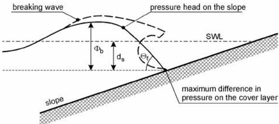
Figure 2.2 Schematization of pressure head on a slope (Source: Klein Breteler et al., 1998)
