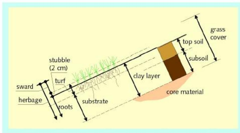
Figure 2.13 Structure and division of a grass cover (Source: Rijkswaterstaat)
