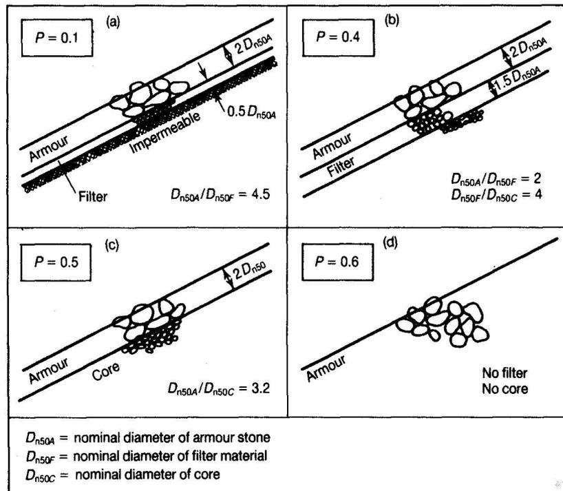
Figure 2.18 Permeability factor  $P$  for the formulae by Van der Meer (1988)
