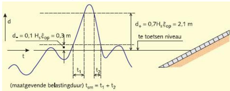
Figure 2.16 Determination of normative duration of loading  $t_{sm}$  (Source: TAW, 2004)
