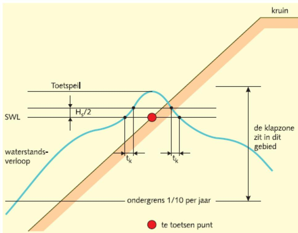
Figure 2.14 Determination of duration of loading in wave impact zone  $t_i$  (Source: TAW, 2004)
