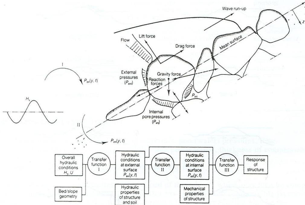
Figure 2.17 A rock system and its responses (Source: CUR, 1995)
