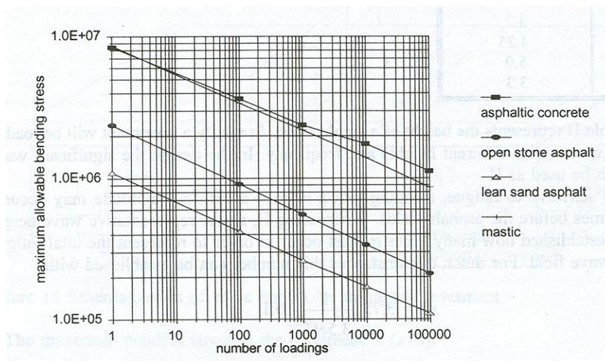
Figure 2.25 Allowable bending stress (Source: Van Herpen, 1998)
