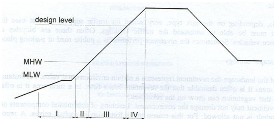
Figure 2.19 Hydraulic loading zones on riverdyke with low foreshore (Source: Van Herpen, 1998)
