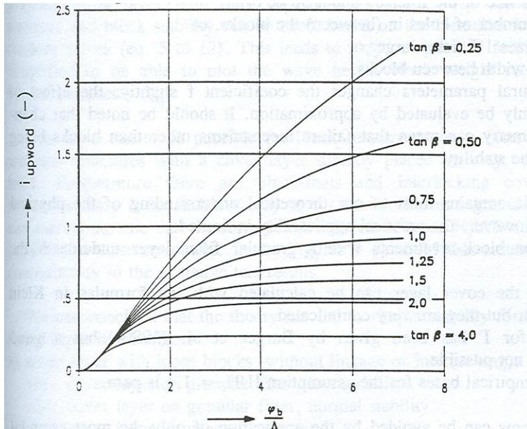
Figure 2.6 Max. upward gradient ( $\tan\beta=\cot\theta$ ). (Source: Klein Breteler & Bezuijen, 1998).
