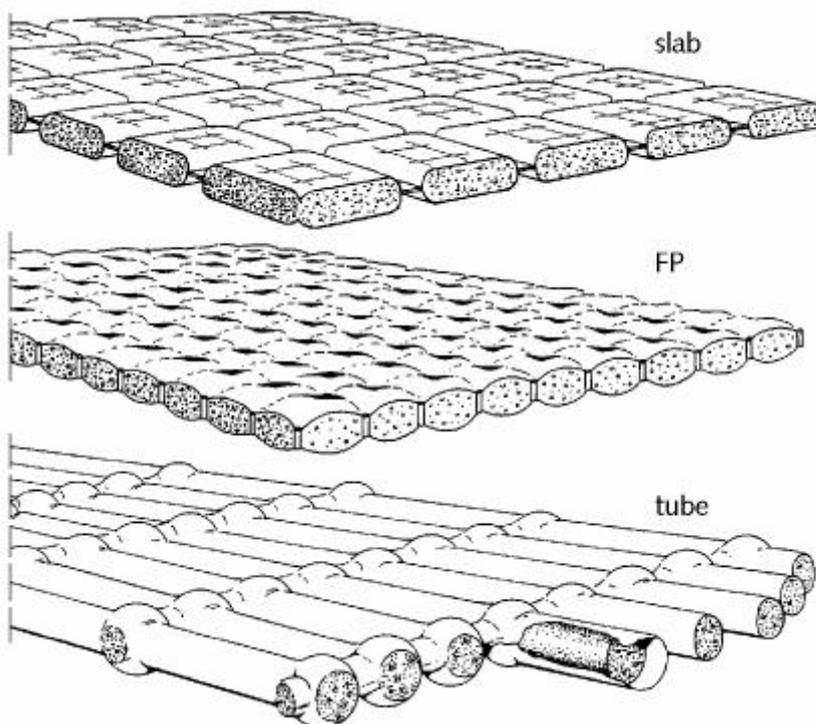
Figure 2.31 Example of concrete-filled mattresses (Source: Klein Breteler et al., 1998)
