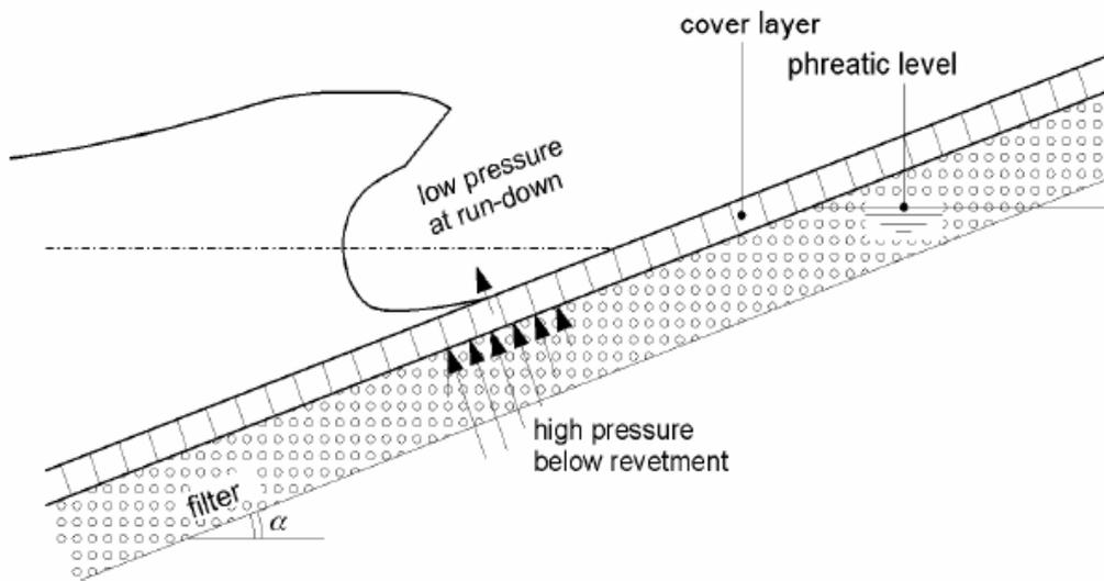
Figure 2.1 Pressure development in a revetment structure (Source: Klein Breteler et al., 1998)
