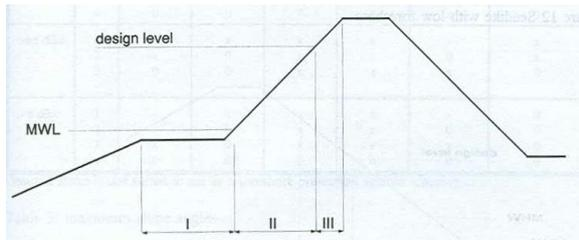
Figure 2.21 Hydraulic loading zones on lake dyke (Source: Van Herpen, 1998)
