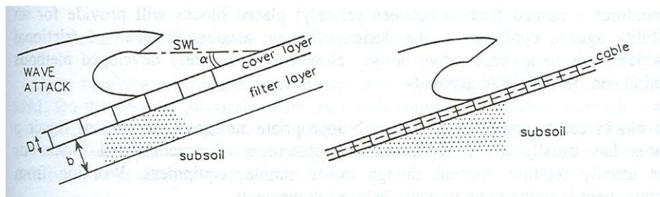
Figure 2.3 Examples of rock revetment structures (cross sections) (Source: Klein Breteler and Bezuijen, 1998)
