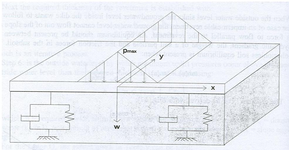
Figure 2.24 Schematization of wave impact on an asphalt revetment (Source: Van Herpen, 1998)
