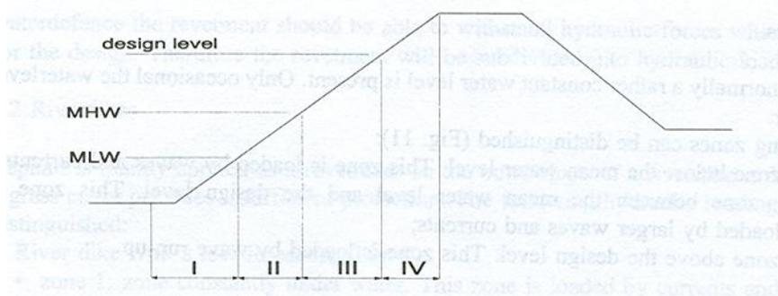
Figure 2.22 Hydraulic loading zones on sea dyke with low foreshore (Source: Van Herpen, 1998)
