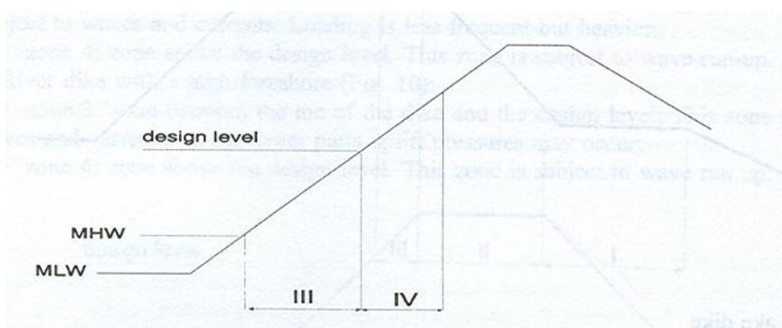
Figure 2.23 Hydraulic loading zones on sea dyke with higher foreshore (Source: Van Herpen, 1998)
