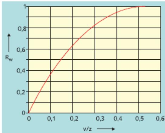
Figure 2.28 Reduction factor  $R_w$  (Source: TAW, 2004)
