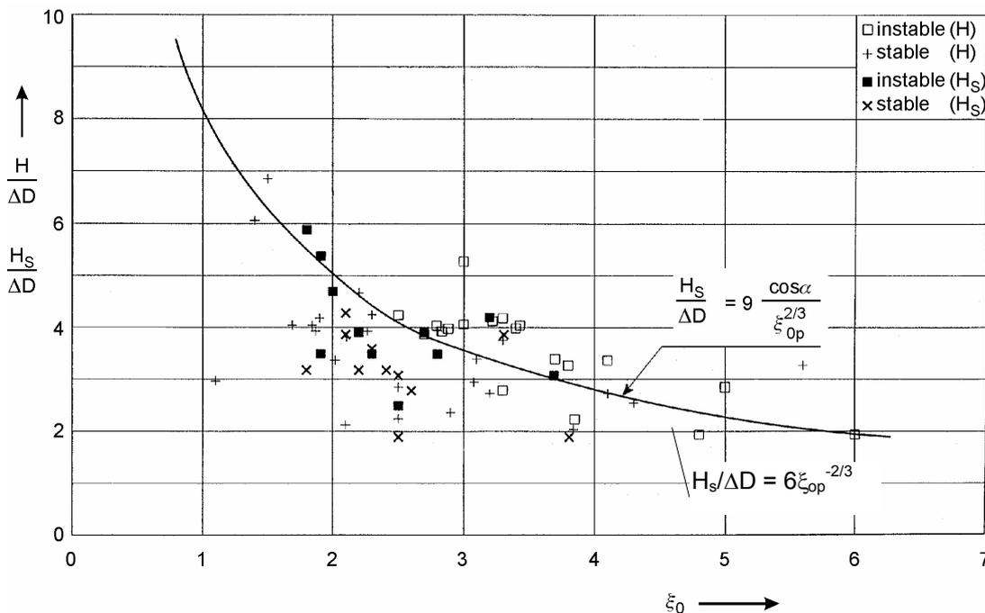
Figure 2.35 Summary of test results ((Ashe 1975) and (Brown 1979)) and design curves (Source: Klein Breteler & Pilarczyk, 1998)
