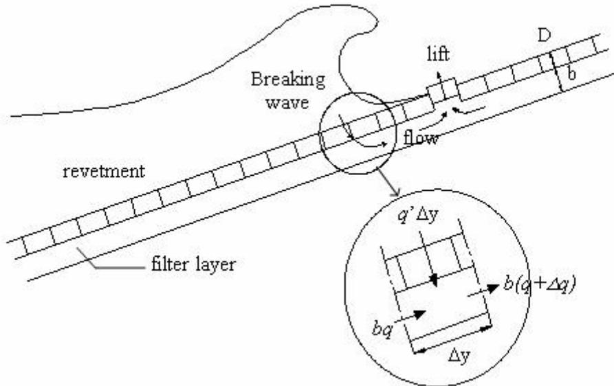
Figure 2.4 Mass balance in filter
