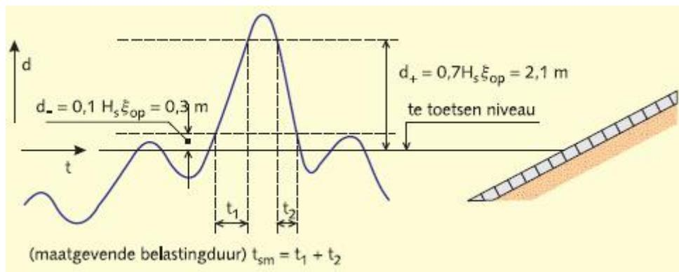
Figure 2.11 Determination of normative duration of loading  $t_{sm}$  (Source: TAW, 2004)
