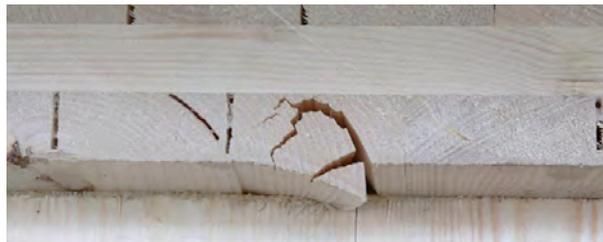
**Figure 2-15: Rolling shear failure**
