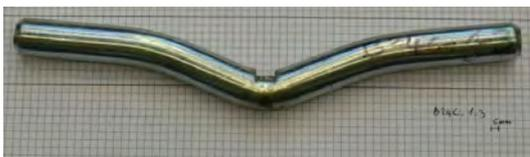
**Figure 7-14: 24 mm hss dowel, test B24C-1-3**
