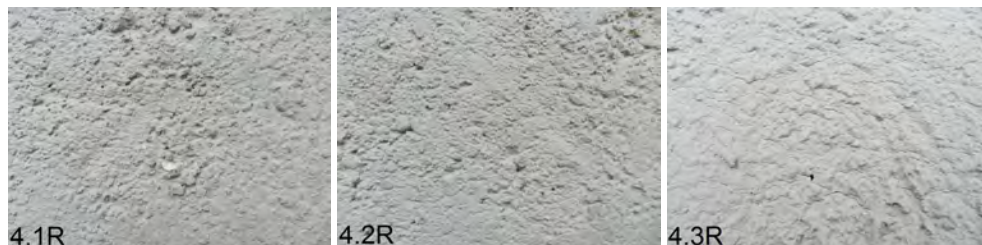
Figure 9.38: Surface cracks in finishing surface of elements 4.1, 4.2 and 4.3 (from left to right, image scale circa 16 x 12 cm)
