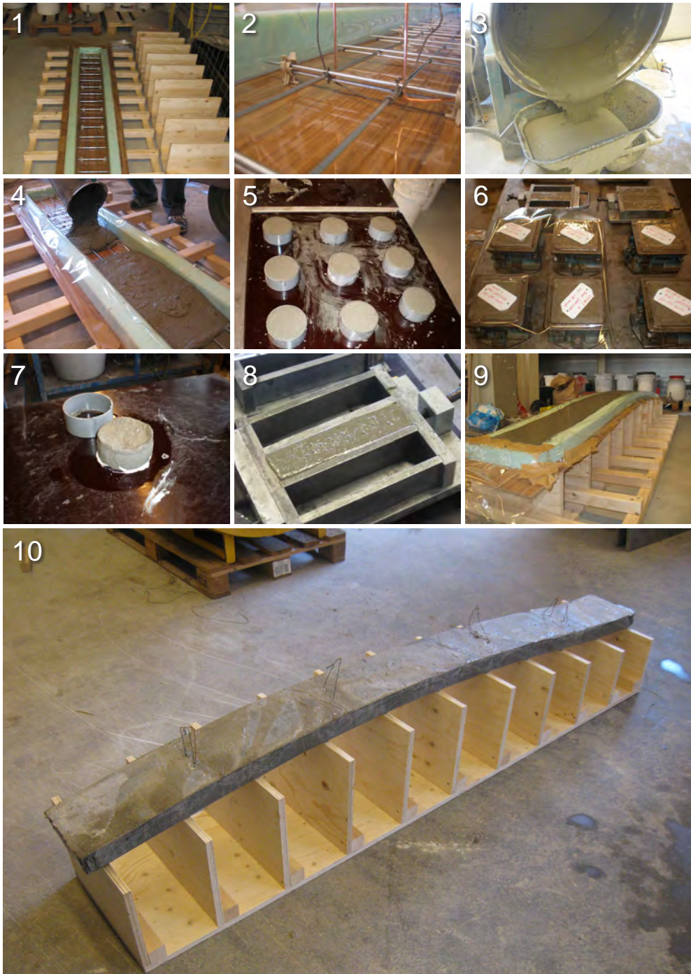
Figure 8.19: Deformation test 1, single-curved element 2.00 \times 0.20 \times 0.05 \text{ m}^3 , \Delta z = 201 \text{ mm} , R_{\min} = 5.00 \text{ m} , slope \theta_{\max} = 5.4^\circ ; deformation at t = 0:50 \text{ h:min} after casting
