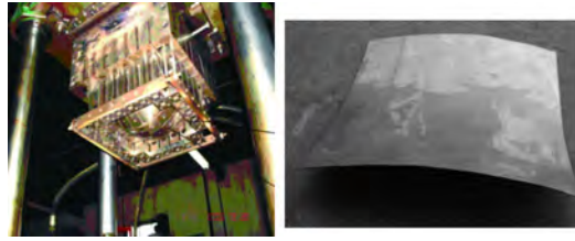
Figure 4.2: Pin-bed mould and sheet of thin metal pressed into saddle shape (taken from Song et al., 2010)
