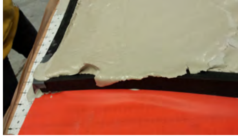
Figure 9.41: Very fluid mixture flows over mould edge after deformation
