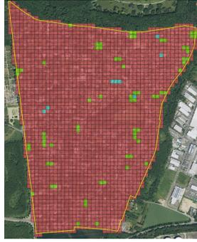
Figure 3.3.: Grid to structure the annotation process; *PV panel* (green), *no PV panel* (red), *unsure* (blue)
