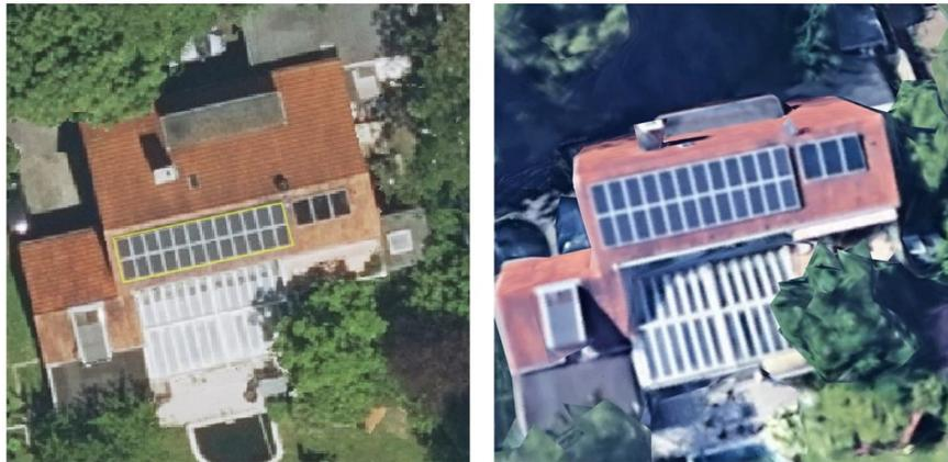
Figure 3.2.: Visual difference between PV panel (yellow polygon) and solar thermal collectors in an aerial image (left) and 3D imagery from Google Earth (right)
