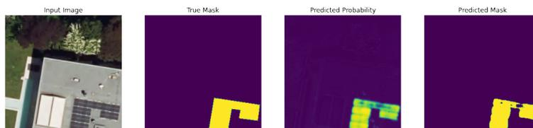
Figure 5.4.: Detection of black PV panels in suburbs
