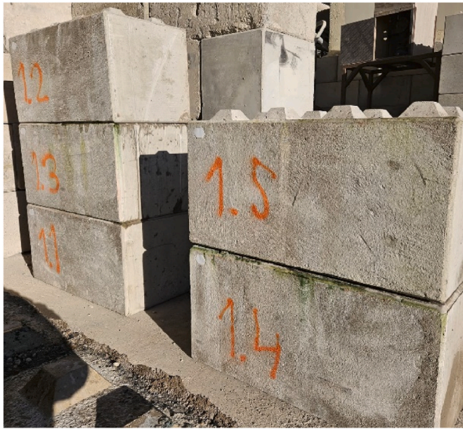
Fig. 4. CEM I-based concrete blocks produced for this experiment. In total 5 units were cast and stored outdoors for approximately 1.5 years.
