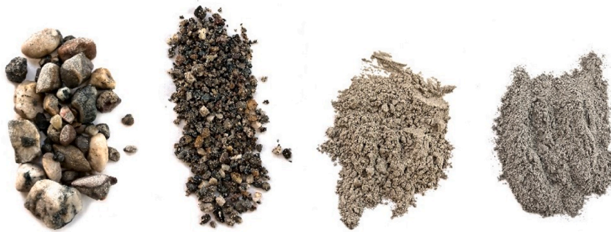
Fig. 5. Fractions obtained through the innovative crushing and separation process. From left to right: secondary gravel, secondary sand, coarse fines 65-250 µm and RCF 0-65 µm.
