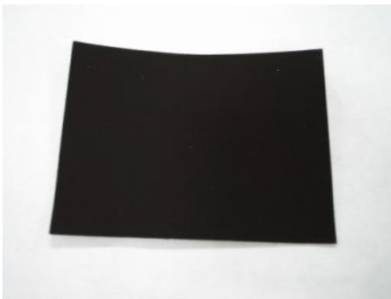
Figure A7. The 0.03 mg/cm 2 20% Platinum on Vulcan - carbon cloth counter electrode was used in LUNA cell experiments. The carbon cloth was cut into 2.54cm*5.08cm rectangles size with a hole for electrodes contact.
