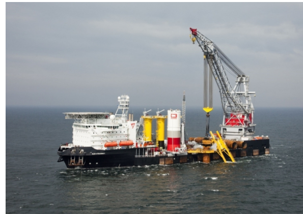
Figure 1.5: Oleg Strashnov installing a monopile [Seaway Heavy Lifting, 2015]
