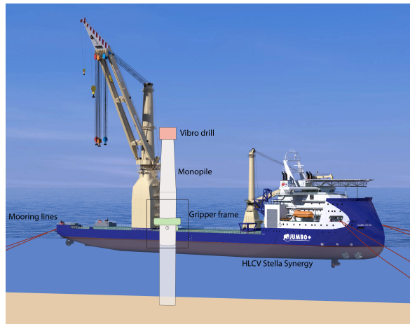
Figure 1: Early driving phase of a monopile installation
