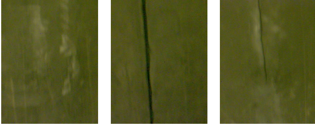
(a) (b) (c) Fig. 3. The collected images:(a) normal image. (b) tear image (c) scratch image
