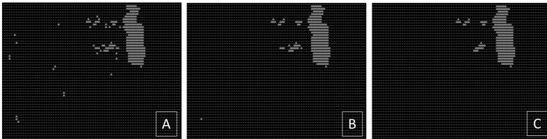
Figure A4: Graph illustrating the cleaning procedure of the cellular automaton algorithm using a set of rules (see text for more details) for the P10 case. White grid cells (zeros) correspond to the ‘populated’ whereas black grid cells (dots) are the unpopulated ones. Shape convergence in this example is achieved after two iterations. Initial and final states in (A) and (C) respectively.
