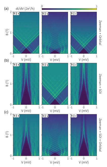
**Figure 4.2:** (a) Numerical simulations of dI/dV as a function of V and B, including the Zeeman and the orbital (Lorentz) effect of the magnetic field. (b) Same as (a), but including Zeeman and SOI instead of the orbital effect, reproducing the anisotropy in Fig. 4.1(e). (c) Same as (b), but including the Zeeman, SOI and orbital effect. The parameters used in (a)-(c) are  $\mu$  = 5.6 meV and  $\Delta V_G$  = -8 meV.
