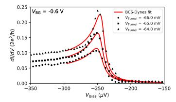
**Figure 5.S4:** Fit (red line) of equation (5.S7) to conductance data from device A (black circles, squares and triangles) for different values of the tunnel gate voltage.
