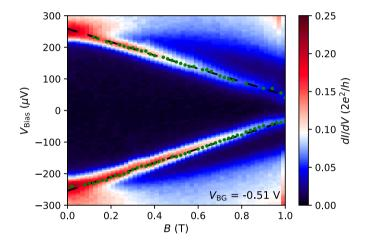
**Figure 5.S8:** Differential conductance as a function of  $V_{\text{Bias}}$  and magnetic field. We apply a linear fit (dashed black lines) to the extracted peak positions (green circles) to obtain the average slope  $\frac{\Delta E}{\lambda B}$ .
