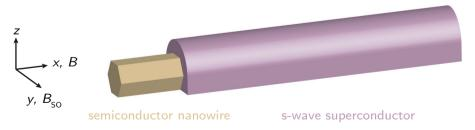
**Figure 2.3: Majorana nanowire** A semiconductor nanowire with strong spin-orbit coupling and a large *g*-factor is covered by a conventional s-wave superconductor. The choice of axes is shown on the left.
