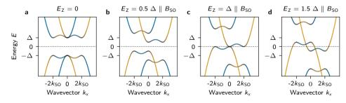
Figure 2.7: Energy spectrum of the Majorana nanowire upon increasing Zeeman energy directed along the spin-orbit field. As the Zeeman field is increased along the direction of  $B_{SO}$ , the energy bands are shifted linearly with  $E_Z$ , resulting in a tilted band structure. The gap closes when the Zeeman field along the spin-orbit direction is equal to gap, and does not reopen at higher fields.  $\mu = 0$  in all panels.
