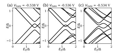
**Figure 5.S15:** Calculated low energy spectrum of the finite size nanowire as a function of Zeeman energy for different values of  $V_{\text{Gate}}$ . Values calculated  $\alpha = 0.1$  eV Å, energy scales in units of  $\Delta$ .
