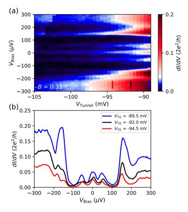
**Figure 5.S17:** (a)  $\mathrm{d}I/\mathrm{d}V$  measured in device A as a function of  $V_{\mathrm{Bias}}$  and  $V_{\mathrm{Tunnel}}$  for  $B=0.35\,\mathrm{T}$  and  $V_{\mathrm{BG}}=-0.37\,\mathrm{V}$ . (b) Line traces at the values of  $V_{\mathrm{Tunnel}}$  indicated by the colored lines in panel (a).
