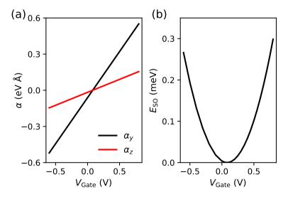
**Figure 5.S2:** (a) Rashba coefficients  $\alpha_y$  and  $\alpha_z$  as a function of  $V_{\rm Gate}$ . At  $V_{\rm Gate}=0.08$  V, the average electric field in the wire goes to zero due to symmetry, leading to vanishing spin-orbit coupling. (b) Calculated  $E_{\rm SO}$  as a function of  $V_{\rm Gate}$ .
