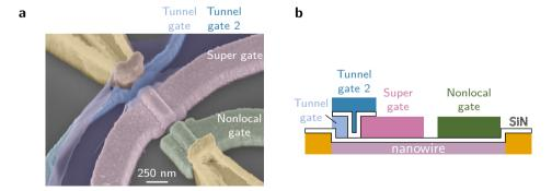
**Figure 7.S6:** Overview of device B. (a) False color tilted view scanning electron micrograph of device B. (b) Side view schematic of device B, cut through the center of the nanowire (not to scale). The layout of the wrap gates is similar to the device discussed in the main text, with the exception of the presence of a second tunnel gate, which overlaps the gap between the tunnel gate and the super gate.
