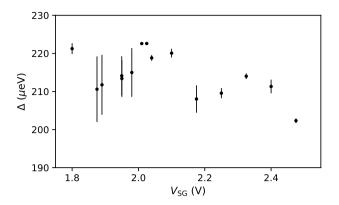
**Figure 5.S5:** Extracted gap  $\Delta$  as a function of  $V_{SG}$  for device B.
