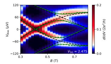
**Figure 5.S12:** Data from device B, showing the differential conductance dI/dV as a function of  $V_{\text{Bias}}$  and B for  $V_{\text{BG}} = 2.475$  V. Green dots indicate the peak positions found using a peak finding algorithm. The fit to the data is shown in green, with the uncoupled asymptotes as the black dashed lines.
