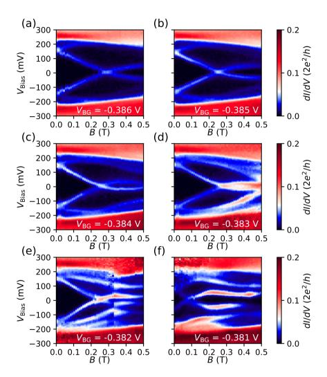
**Figure 5.S18:** Differential conductance as a function of  $V_{\text{Bias}}$  and magnetic field. Although the lowest energy state stays near zero over an extended magnetic field range for some gate voltages, this behavior is not robust.
