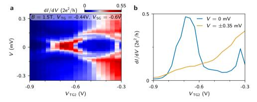
Figure 6.S5: Dependence of the ZBP in device A shown in Fig. 6.3 on the additional tunnel gate. (a) As the voltage on the additional tunnel gate  $V_{\rm TG2}$  (see Fig. 6.3a) is varied, the subgap state comes down from finite energy, crosses zero energy to form a ZBP, and then splits off again, analogous to the dependence on the primary tunnel gate (Fig. 6.3e). (b) Horizontal linecuts of  $\bf a$  at zero bias (blue) and the above-gap conductance, taken as the average of -0.3 and 0.3 mV.
