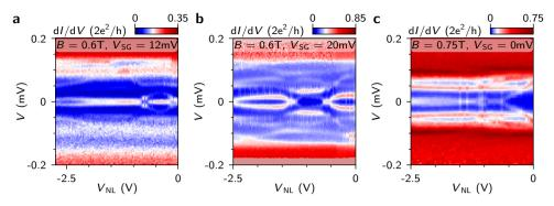
**Figure 7.S5:** Additional nonlocal gate dependences. (a,b) Nonlocal gate dependence of the ZBP in Fig. 7.4 showing peak splitting modulation at  $V_{\rm SG}=12\,\rm mV$ ,  $V_{\rm SG}=20\,\rm mV$  and  $V_{\rm TG}=-162\,\rm mV$ ,  $V_{\rm TG}=-137\,\rm mV$  in a,b respectively. (c) At  $B=0.75\,\rm T$  we observe two small peak splitting oscillations, after which the ZBP fully splits towards the gap edge.  $V_{\rm TG}=-150\,\rm mV$ .
