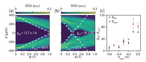
**Figure 5.S11:** (a,b) Simulated nanowire spectrum as a function of magnetic field including orbital effects. (c) Extracted  $g_{\text{eff}}$  (black circles) and  $g_{\text{spin}}$  (red squares) as a function of  $V_{\text{Gate}}$ .
