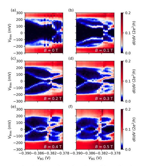
Figure 5.S19: Differential conductance as a function of  $V_{\rm Bias}$  and  $V_{\rm BG}$ . We find some stable ZBPs for certain ranges in back gate voltage at specific fields, but this is only true for fine tuned parameters.
