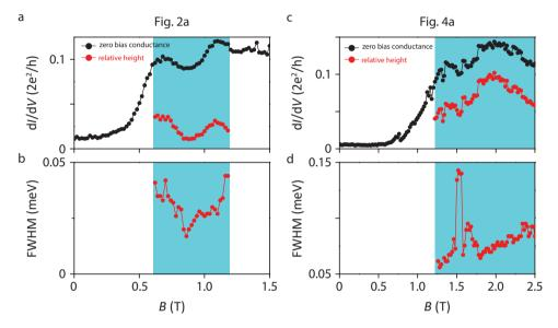
**Figure 3.S4: Zero-bias peak height and width. (a)** The absolute and the relative height of the zero-bias peak extracted from main text Figure 3.2a. The difference between the absolute and the relative height is the subgap conductance around zero bias for each magnetic field. **(b)** The full width at half maximum (FWHM) of the zero-bias peak extracted from main text Figure 3.2a. **(c,d)** Same as **a** and **b** but for the zero-bias peak from main text Figure 3.4a.
