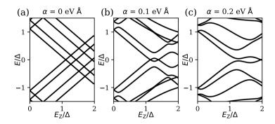
Figure 5.S14: Calculated low energy spectrum of the finite size nanowire as a function of Zeeman energy for different values of  $\alpha$ . Values calculated for  $V_{\text{Gate}}$  = -0.536 V, which is also used in main text figure 5.4(d). All energy scales are in units of the superconducting gap  $\Delta$ .
