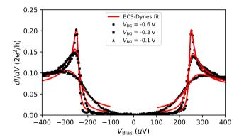
Figure 5.S6: Fit (red line) of equation 5.S7 to conductance data from device D (black circles, squares and triangles) for different  $V_{\rm BG}$  at similar junction transparencies. The dissipation broadening sharply decreases for more negative gate voltages.
