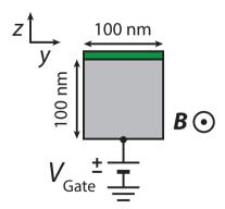
Figure 5.S13: Schematic cross-section of the geometry used to simulate the finite nanowire system. A potential  $V_{\rm Gate}$  is applied to the bottom facet, while the potential at the top facet is fixed by the work function difference between the two materials. The magnetic field is applied in the x-direction, along length of the nanowire.
