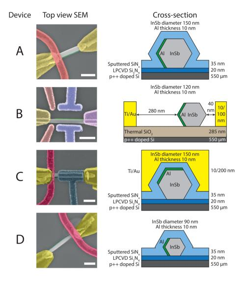
**Figure 5.S1:** SEM images and schematic cross-sectional views of the devices used as part of this research. Data from devices A and B is presented in the main text. Data from devices C and D is presented in the supplement for completeness. Note that the data for device B is obtained by changing the voltage on the side gate ( $V_{SG}$ ), shown in blue in the SEM image. Scale bar is 500 nm.
