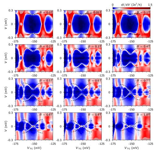
Figure 7.S1: Extraction of the dot ABS parameters in Table 7.S1. The colormap shows the spectrum of the dot ABS upon variation of  $V_{\rm TG}$  at increasing magnetic fields. The black dotted lines show the ABS spectrum obtained from the model. We note that we observe some small deviations between the model and the data since we do not take interaction with subgap states underneath the super gate into account here.  $V_{\rm SG} = 22\,\mathrm{mV}$ ,  $V_{\rm NL} = 0\,\mathrm{V}$  in all panels.
