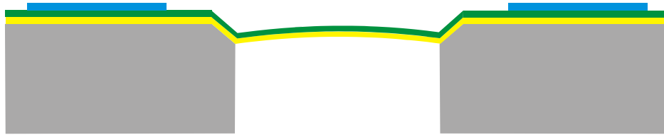
Figure 8 Cross section of a silicon version of the strain sensor.
