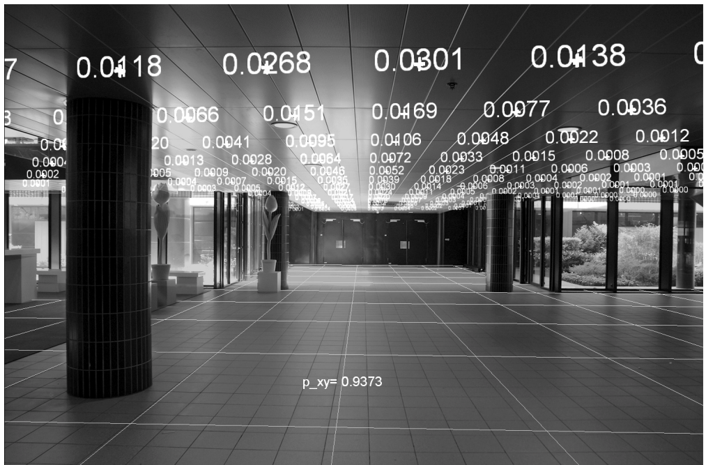
Fig. 2.20 Space corresponding to the perception computation shown in figure 2.19, where l_o=1.5\text{m} ; the resulting degree of perception of the ceiling is P_{x,y} \cong 0.94 .
