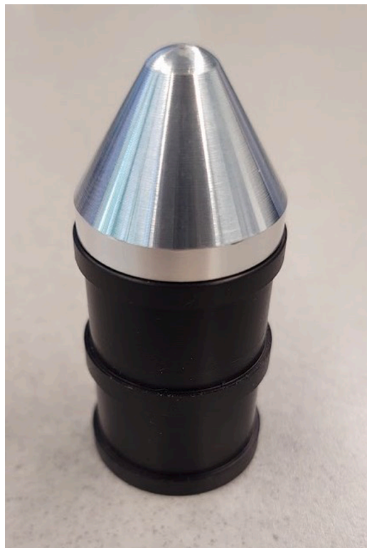
Fig. 4. The aluminium projectile screwed into a POM rear section.
