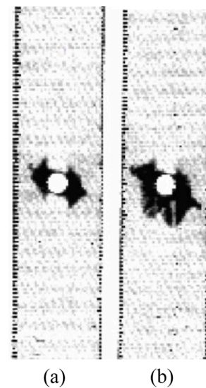
Fig. 24. C-scan images for specimens 37 paused and scanned at 20% strain increase (a) and 32 paused, impacted and scanned at 20% strain increase (b).
