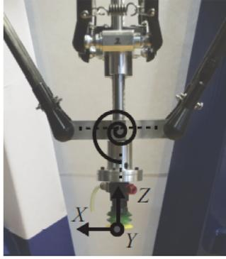
**Fig. 4.** It was found that structural compliance in the end-effector assembly of the Heli4 manipulator is significant and that this can be represented by a rotational stiffness of 500 Nm/rad and a linear stiffness of 1.3e5 N/m around the Y-axis located at the center of the lower traveling plate (center of schematic spring).
