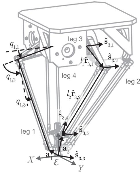
Fig. A.1. Examples of the various vectors that are used in the description of the unit twists and unit wrenches of the Heli4 manipulator.
