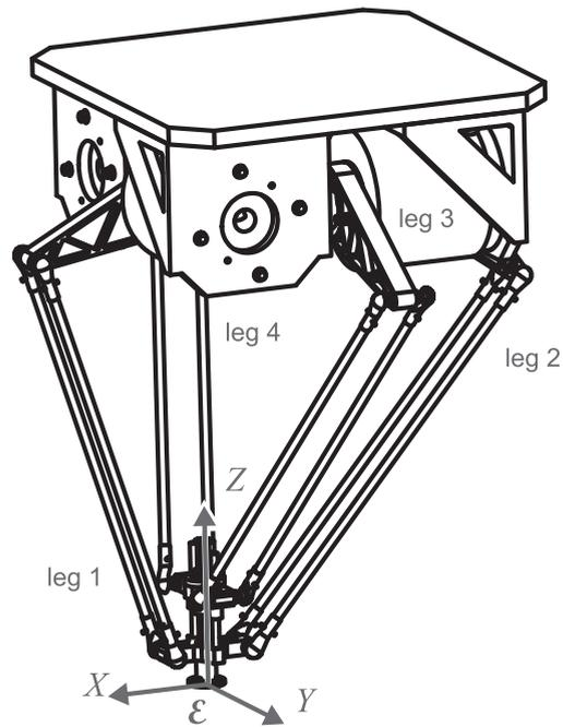
**Fig. 1.** The Heli4 manipulator is modeled as a 4-RR1RR robot. All twists, wrenches and matrices are expressed in the Cartesian end-effector reference frame  $\mathcal{E}$ .
