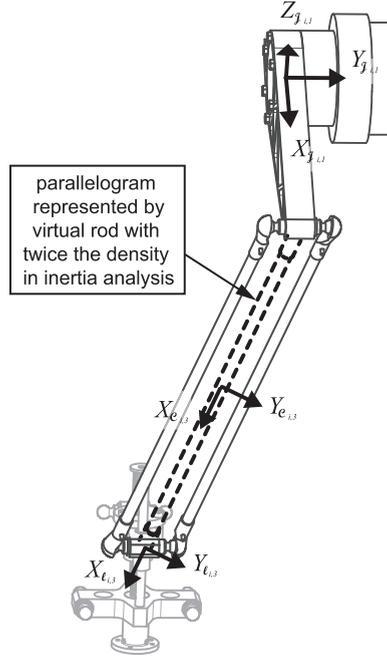
**Fig. 3.** The inertia of the first link and the actuator are expressed in reference frame  $\mathcal{J}_{i,1}$ . To represent the inertia of the parallelogram it is modeled as a single rod, positioned midway between the two parallel rods, with double the mass density.
