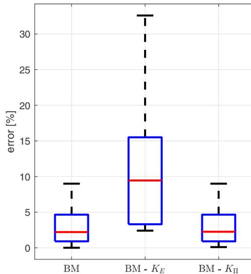
**Fig. E.1.** Boxplots of all errors in percentages for the benchmark model (BM), BM excluding structural compliance of the end-effector assembly (BM- $K_E$ ), and BM excluding structural compliance originating in the links of the parallelogram (BM- $K_{\Pi}$ ).
