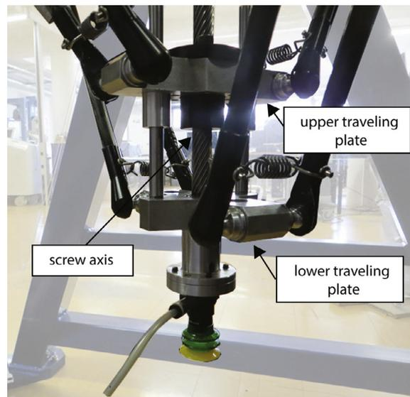
**Fig. 2.** The end-effector assembly of the Heli4 manipulator facilitates the rotational motion of the end-effector by transforming a differential motion of the two traveling plates to rotational motion using a screw axis. In this paper it was found that friction prevented this rotational motion from being excited, so that in this paper the end-effector assembly is considered as a single body.
