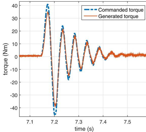
**Fig. B.1.** It was observed during the verification tests that there was a loss a factor of 0.82 between the demanded and generated torque, here demonstrated for motor 1 with  $k_d = 2000$  Nm/rad for the step input in the X-direction.
