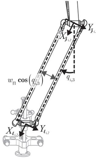
**Fig. C.1.** To model the structural compliance of the two rods that are part of the parallelogram, they are assumed to share the rotation points located in the origins of reference frames  $J_{i,2}$  and  $\ell_{i,2}$ .
