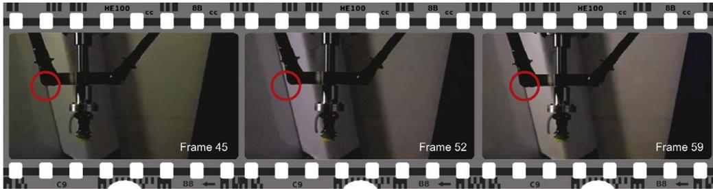
**Fig. 5.** A series of frames from one of the high-speed video for the step response in X-direction with a actuator stiffness of 2000 Nm/rad. The frames capture one oscillation going from left to right and back, which can for example be observed in the red circles by the relative motion of the end-effector with respect to the background.
