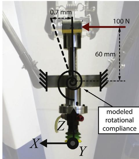
Fig. D.1. One aspect of the structural compliance in the end-effector was measured using a displacement measurement under a loading of 100 N.
