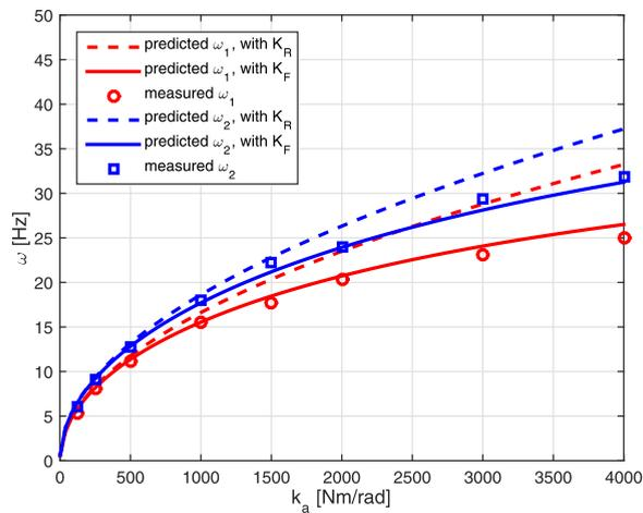
**Fig. 6.** The predicted values for the two lowest natural frequencies, using either the rigid-body stiffness model or the flexible-body stiffness model, as well as the measured natural frequencies as a function of actuator stiffness values.
