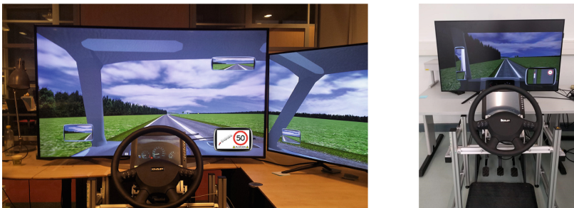
Fig. 1. Left: Setup for Experiment 1 (65- and 49-inch screen). Right: Setup for Experiment 2 (49-inch screen.) The instrument cluster was shown on a 12-inch screen behind the steering wheel.
