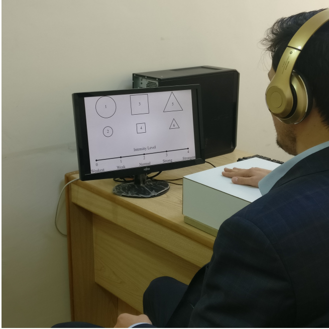
Fig. 3. Experiment setup where subject’s right hand rests on the apparatus. The screen shows the stretch intensity scale and the shapes and sizes used in the experiments.
