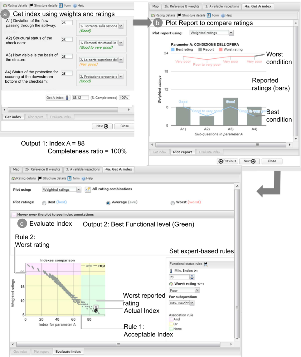
Figure 5.9: Outputs from the evaluation module: a) Index and a completeness ratio indicating the reported ratings. b) Report plot to compare ratings with reference conditions. c) Functional category of the parameter according to expert-based rules
