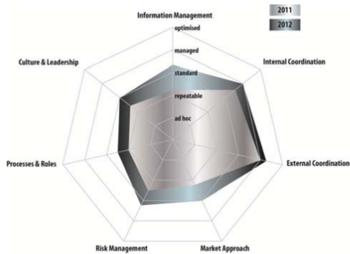
Figure 5.1: An example of IM3 maturity model. This example is an assessment of the asset management maturity in two different years. In 2012, the organization showed a significant improvement in every maturity dimension (Volker et al., 2013).
