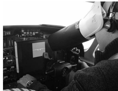
Figure G.1. The field-of-view constraining hood that was used during the in-flight tracking tasks (a) and one of the pilots performing an in-flight tracking task while wearing the hood (b).
