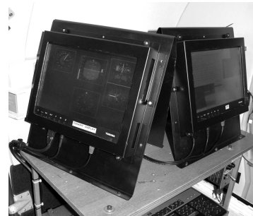
Figure D.2. The two Toshiba M700 touch-screen tablet notebooks in their mounts in the Cessna Citation II laboratory aircraft ( citefis at left, citecs at right).
