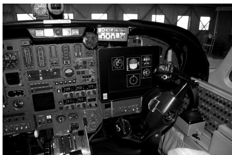
Figure 6.17. The Cessna Citation II laboratory aircraft cockpit.
