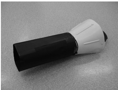
Figure G.1. The field-of-view constraining hood that was used during the in-flight tracking tasks (a) and one of the pilots performing an in-flight tracking task while wearing the hood (b).
