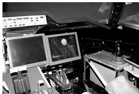
Figure 6.18. The SIMONA Research Simulator cockpit.
