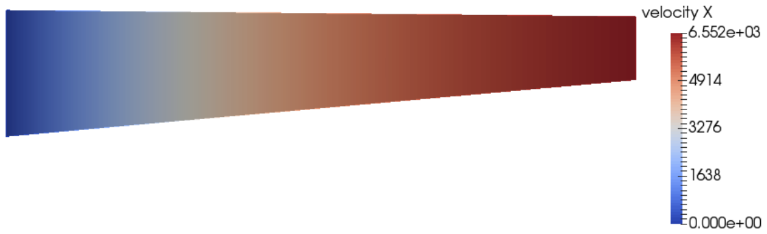
Figure 14: The horizontal velocity in the FS solution for the ice shelf ramp.
