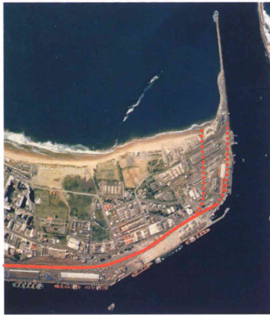
figure 7-4: existing railroad with extension options;
