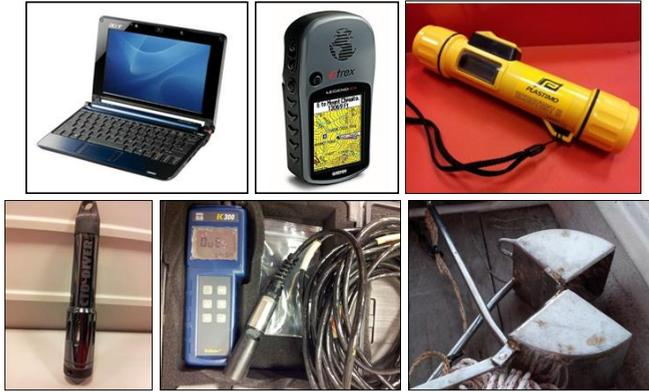
Figure 3.2: Equipment used in conducting filed survey (from top left: netbook, GPS, handheld depth sounder, diver, conductivity meter, and Van Veen Grab)
