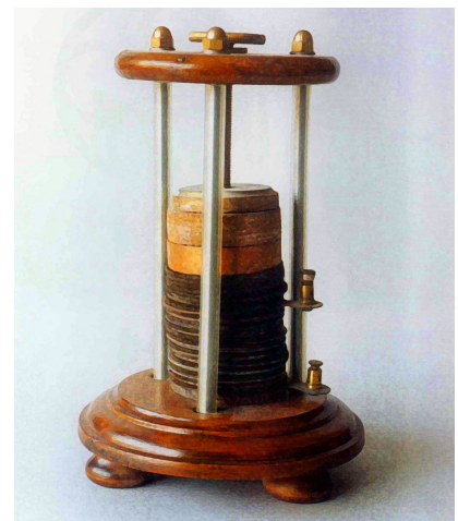
Figure C.2: Alessandro Volta pile, the first direct current battery.
