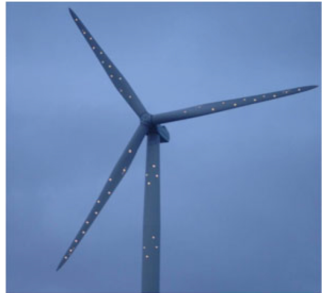
Figure 6. Example of turbine instrumentation with reflective markers for photogrammetry or laser interferometry (Ozbek and Rixen, 2013).
