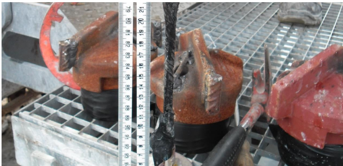
Figure 2-1: Sacrificial drill bits of Type B micropiles as applied at the Drachtsterweg (Picture B. Niezen)
