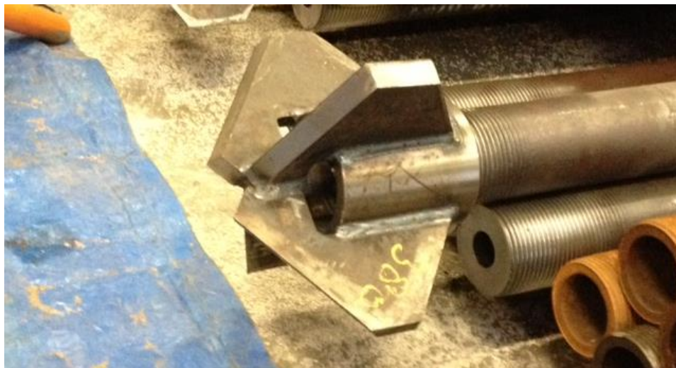
Figure 2-2: Drill bit of a Type C micropile as applied at the Drachtsterweg (Pictures Ir. J. Kimenai)
