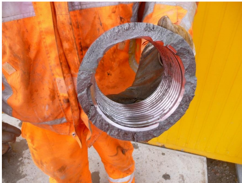
Figure A-6: Failed coupling of a micropile at the Drachtsterweg, Leeuwarden (Pictures Ir. Kimenai)
