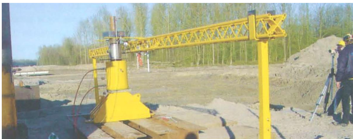
Figure 2-9: Example of test setup in which the measurement equipment is separated from the test construction (CUR236, 2011)
