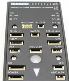
Figure 7. The HobbyKing HKPilot32 micro-controller.
