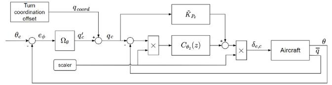
Figure 6. Pitch control scheme of the UAV. The variables  $\theta$ ,  $\theta_c$  are the pitch and commanded pitch angle, while the variables  $\bar{q}$ ,  $q_c$  are the pitch rate and commanded pitch rate. The commanded elevator is  $\delta_{e,c}$ .
