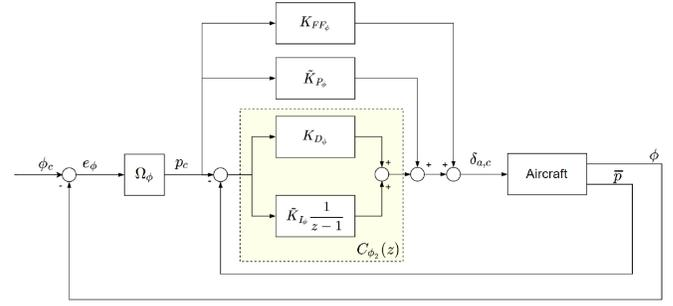
Figure 5. Roll control scheme of the UAV. The variables  $\phi$ ,  $\phi_c$  are the roll and commanded roll angle, while the variables  $\bar{p}$ ,  $p_c$  are the roll rate and commanded roll rate. The commanded aileron is  $\delta_{a,c}$ .
