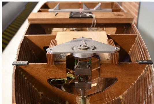
Figure 4.3: The rudder angle gauge, dynamometers and clamp used for the tests.
