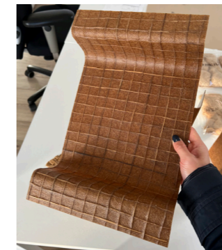
Figure 48: Compressed sheet of bamboo fibers and long fibers from Bambooder.
