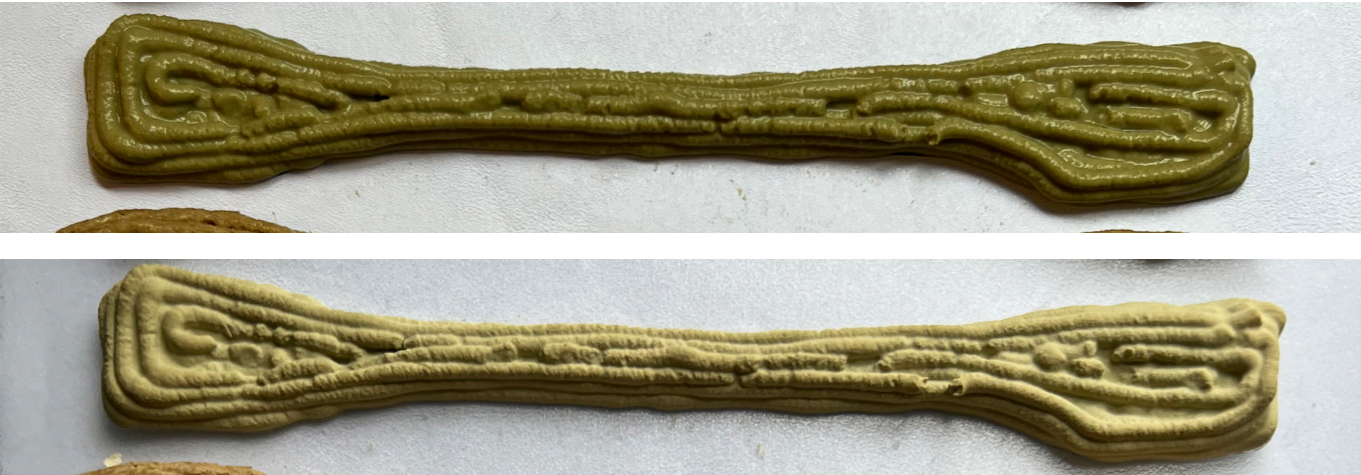
Figure 140: Mixture result with tapioca starch before and after drying
