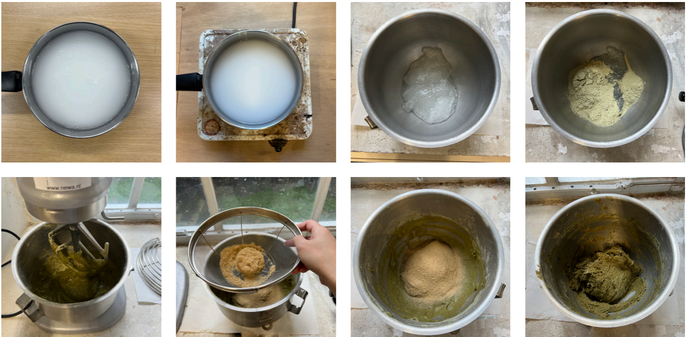
Figure 178: Mixture procedure with clay mixer.
