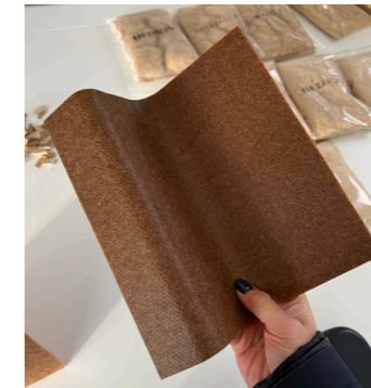
Figure 46: Bamboo fibers with cork from Bambooder.
