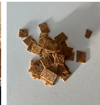
Figure 49: Flakes made with pressed bamboo fibers and resin from Bambooder.
