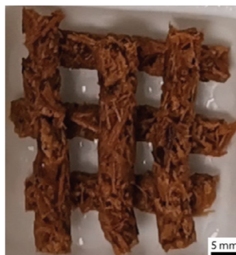
Figure 79: Extrusion of mycelium-enriched bamboo fibres-chitoan pastes (Soh et al.,2020).
