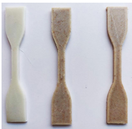
Figure 78: Images of the 3D printed species (left to right): ABS, ABS-bamboo, ABS-bamboo modified (Gama et al., 2021).
