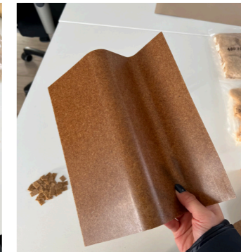
Figure 47: Compressed sheet of bamboo fibers from Bambooder.
