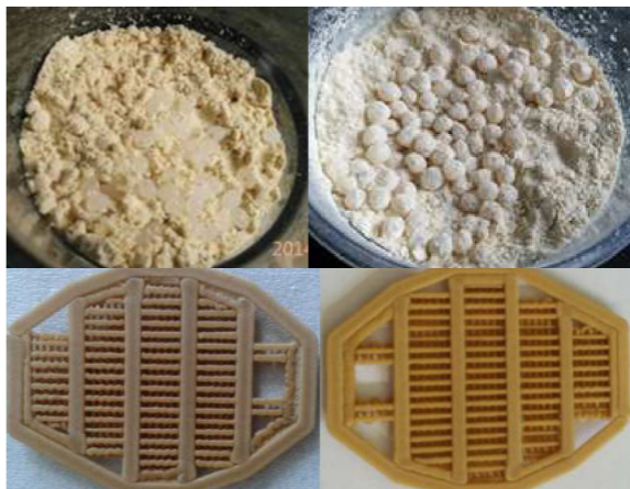
Figure 80: Premixing bamboo powder with PLA and comparison of different adding proportion (Zhao et al.,2015).
