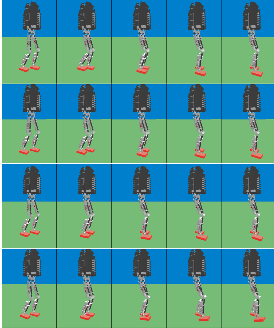
Figure 7.2: From left to right a graphical representation of the state of the robot for t = 0.0 s, t = 0.1 s, t = 0.2 s, t = 0.3 s, and t = 0.4 s is shown for a forward step. The different controllers are shown from top to bottom: a) MPC - Minimum torque cost function, b) MPC - Minimum torque change cost function, c) Minimum jerk controller, and d) Foot trajectory controller. Note that the images are mirrored for clarity.
