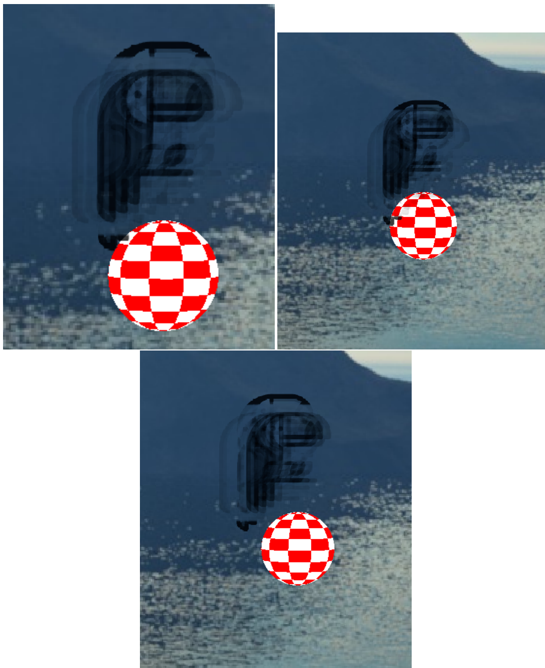
Figure 5.2: An icon seen from different positions within the eye box. The toucan is always visible, and moves similarly to the ball, a stand in for a real object. If not focused on, the toucan should seem blurry
