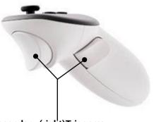
Primary (left) and Secondary (right) Triggers: These analogue input methods are primarily used to interact with objects within the virtual environment. They are used to select/deselect, move, equip/unequip and rotate objects in an environment.
