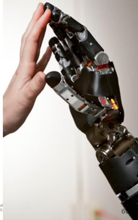
Figure 6.2: Modern prosthetic arms use EMG sensors to control the grip of their prosthetic limbs (Air Force Medical Service, 2015).
