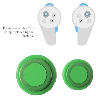
Figure 7.5: Modules come in two sizes Large, 8 cm and small, 6 cm.
