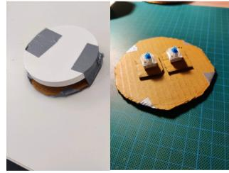
Figure 7.19: Prototype of the arm bands and the button module with the keyboard switch underneath (extreme right).
