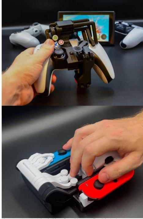
Figure 2.15: DIY 3D - Printed add-ons for making controllers (PlayStation 5 controllers (top), Nintendo Joycons (below)) (Akaki Controllers, n.d.).
