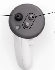
Action Buttons (XYAB buttons): Two on each controller; these buttons can be mapped to any action within the game. Unlike conventional controllers, their usage in the virtual world has been significantly reduced to make minute interactions (unequip/equip, pause game, etc.).
