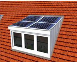
Figure 5.8: Close-up of small solar dormer (Ow III)
